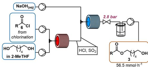
**Scheme 3** Flow scheme for the acylation of 1,6-hexanediol in 2-MeTHF (3 equiv., 2.5 M) at 100 °C for 4 min with fatty acyl chloride **6** (1 equiv., crude from previous reaction) and subsequent neutralisation with aqueous NaOH (1 M, 4.4 equiv.) at 0 °C for 2 min to obtain monoester **3**.
