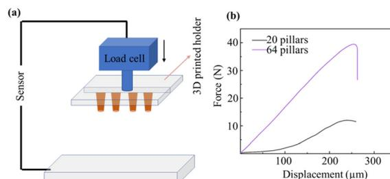
**Fig. 4** A schematic of the compression force measurement and resulting force-displacement curves. (a) The compression force measurement setup with a maximum load cell of  $50 \text{ N}$ , (b) force vs. displacement curves for different numbers of pillars.
