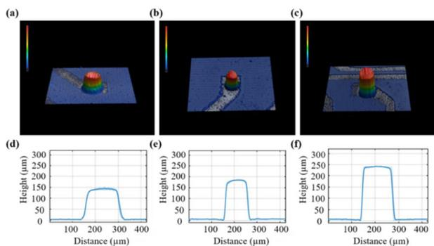
**Fig. 2** 3D profile analysis of patterned microelectrodes. (a), (b) and (c) show 3D profiles of exemplary microelectrodes produced from different epoxy-based pillars' layers captured via a 3D laser scanning confocal microscope. The scale bar for the height is shown at the top left of each image. The profiles were averaged from 6 directions and plotted in (d), (e), and (f).
