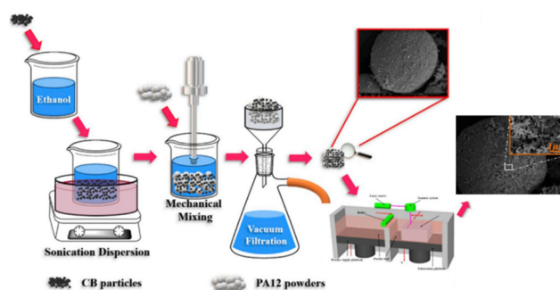
Fig. 13 Schematic illustration of the two-step approach for producing carbon black/polyamide 12 composites with a 3D segregated conductive network. 93
