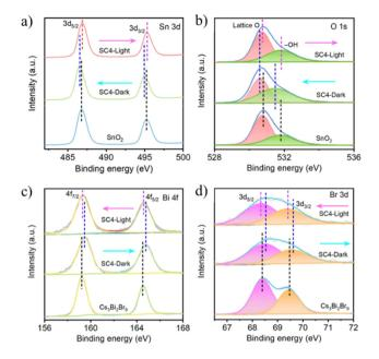
Fig. 3 High-resolution XPS spectra of (a) Sn 3d, (b) O 1s, (c) Bi 4f, and (d) Br 3d for SnO<sub>2</sub>, Cs<sub>3</sub>Bi<sub>2</sub>Br<sub>9</sub>, and SC4 obtained in the dark and under UV light irradiation, respectively. Reprinted with permission from ref. 66. Copyright 2023 American Chemical Society.
