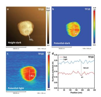
Fig. 4 (a) AFM and (b) KPFM images of TF in the absence of light. (c) image of TF under UV light illumination at 365 nm. (d) Corresponding surface potential profiles. Reprinted with permission from ref. 69. Copyright 2022 Wiley-VCH.
