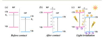
Fig. 2 Graphical illustration of the charge migration process of S-scheme heterojunctions. (a) before contact; (b) after contact; and (c) photogenerated charge carrier transfer under light irradiation.
