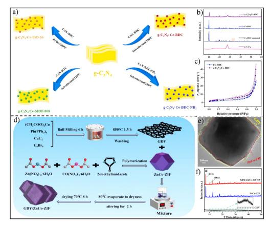
Fig. 8 (a) Synthesis process of  $g-C_3N_4/Ce-MOF$ . (b) XRD patterns of  $g-C_3N_4$ . Ce-BDC, and  $g-C_3N_4/Ce-BDC$ . (c)  $N_2$  adsorption—desorption isotherms of Ce-BDC and  $g-C_3N_4/Ce-BDC$ . Reprinted with permission from ref. 43. Copyright 2023 Elsevier. (d) Schematic for the preparation of GDY/ZnCo-ZIF. (e) TEM image of GDY/ZnCo-ZIF. (f) XRD spectra of GDY, ZnCo-ZIF and GDY/ZnCo-ZIF. Reprinted with permission from ref. 96. Copyright 2023 Elsevier.
