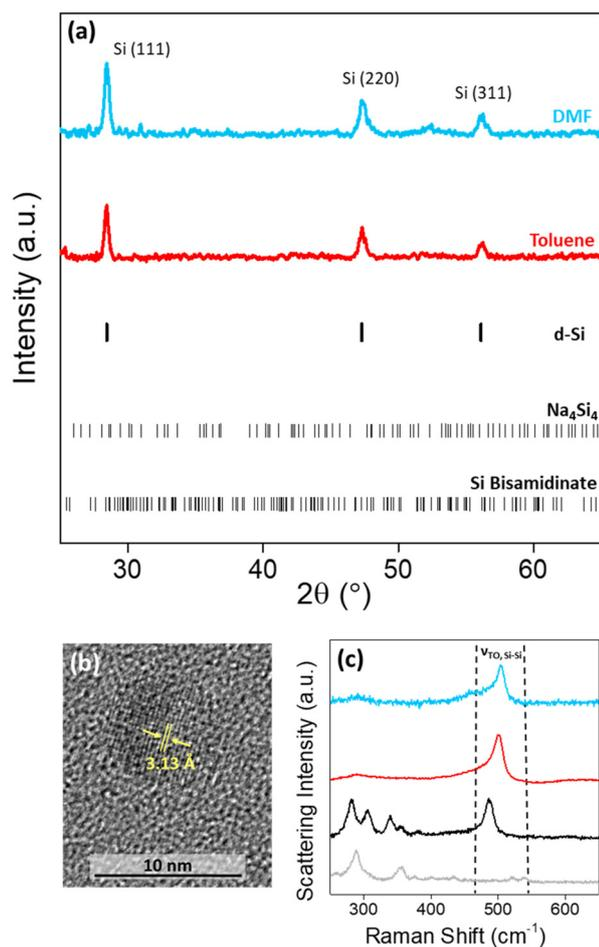
**Fig. 3** (a) Powder XRD patterns of product produced in (blue) DMF and (red) toluene with Bragg peak positions plotted for diamond cubic Si,  $\text{Na}_4\text{Si}_4$  and silicon bisamidinate precursors. (b) HRTEM image of an individual particle produced in DMF showing lattice fringes corresponding to  $d$ -spacing of (111) cubic Si plane. (c) Raman spectra of (black) silicon bisamidinate, (grey) sodium silicide, and particles produced in (blue) DMF and (red) toluene.
