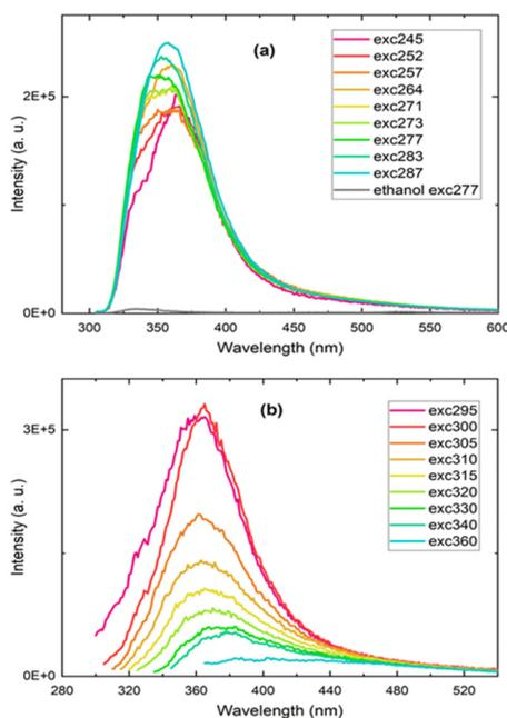
**Fig. 5** Photoluminescence emission spectra of silicon nanoparticles prepared in toluene and further dispersed in ethanol. The photoluminescence spectra were obtained with different excitation wavelengths: (a) excitation from 245 nm to 287 nm (b) excitation from 295 nm to 360 nm. The PL emission spectrum of ethanol alone is shown in (a) for comparison.
