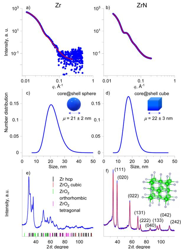
**Fig. 5** Size and crystallinity investigations of Zr NPs (left column) and ZrN NPs (right column): (a and b) SAXS data with fitting curves; (c and d) size distribution obtained from SAXS fitting using a spherical model for Zr and cubic model for ZrN; (e and f) XRD patterns. Red curves in a, b, f are fits to the experimental data.
