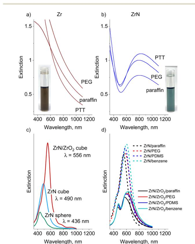
**Fig. 9** Measured UV-Vis spectra of (a) Zr ( $50 \mu\text{g ml}^{-1}$ ) and (b) ZrN ( $30 \mu\text{g ml}^{-1}$ ) nanofluids in PEG, paraffin and PTT (insets show vials with Zr/paraffin and ZrN/paraffin nanofluids). FDTD simulated extinction spectra of a single NP: (c) ZrN sphere (22 nm diameter) vs. ZrN cube (22 nm edge length) vs. ZrN/ZrO<sub>2</sub> core@shell cube (18 nm core and 2 nm shell); (d) ZrN and ZrN/ZrO<sub>2</sub> core@shell cube NPs in different liquids.
