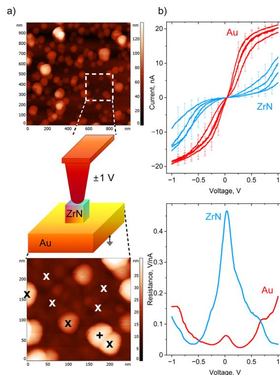
Fig. 8 (a) Different scan size AFM images of ZrN NPs on Au with a scheme of the  $I$ - $V$  measurements, "x" designates the spots used for obtaining the  $I$ - $V$  curves; (b) site-selective  $I$ - $V$  curves measured by a conductive tip on "x" spots and the averaged resistance ( $dV/dI$ ).
