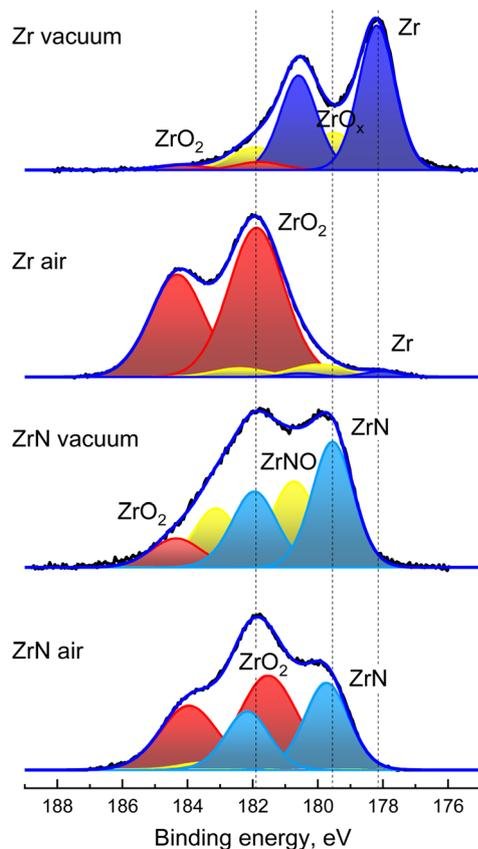
Fig. 6 XPS Zr 3d spectra of Zr and ZrN NPs acquired immediately after sample preparation without breaking vacuum and after one day storage in air.
