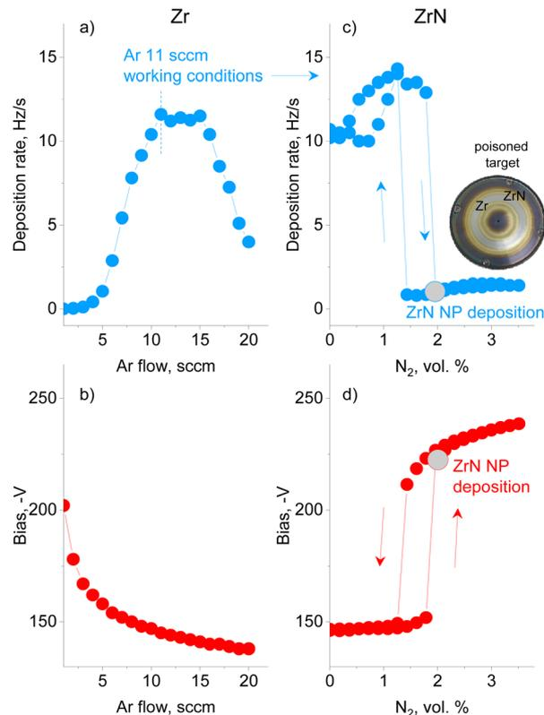
**Fig. 2** The deposition rate of NPs and dc bias at the magnetron for: (a and b) sputtering of Zr in Ar under different flow rates; (c and d) sputtering of Zr in Ar/N<sub>2</sub> (the Ar flow rate is fixed at 11.0 sccm and the N<sub>2</sub> flow rate is increased stepwise). The magnetron current is fixed at 500 mA. The gray symbols designate the working conditions for the synthesis of ZrN NPs. The inset shows the top view of the Zr target after many runs of reactive sputtering.
