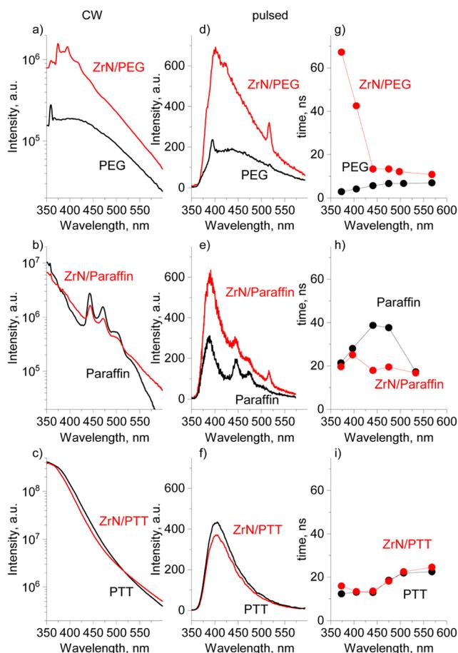
**Fig. 10** Photoluminescence of ZrN nanofluids vs. blank solvents: (a–c) PL spectra at CW excitation ( $\lambda_{\text{exc}} = 325$  nm); (d–f) PL spectra at pulsed excitation ( $\lambda_{\text{exc}} = 355$  nm, 200 fs pulse length, 400 nJ per pulse); (g–i) average PL decay times at different emission wavelengths.
