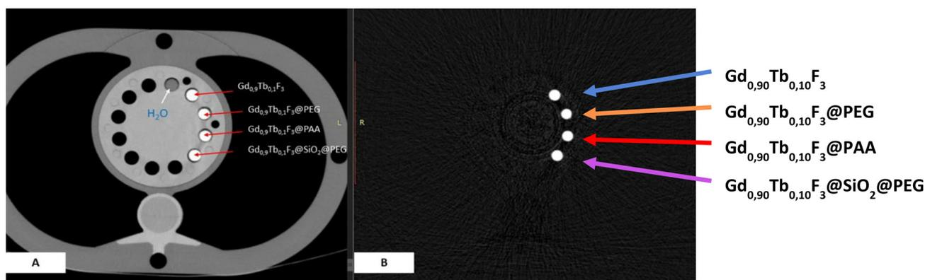
**Fig. 7** (A) Conventional SPCCT imaging of a phantom containing colloidal suspensions of normal, PEG modified, PAA modified and  $SiO_2@PEG$  modified NCs in water (0.5 M). (B) Same phantom with color gadolinium K-edge imaging using SPCCT.
