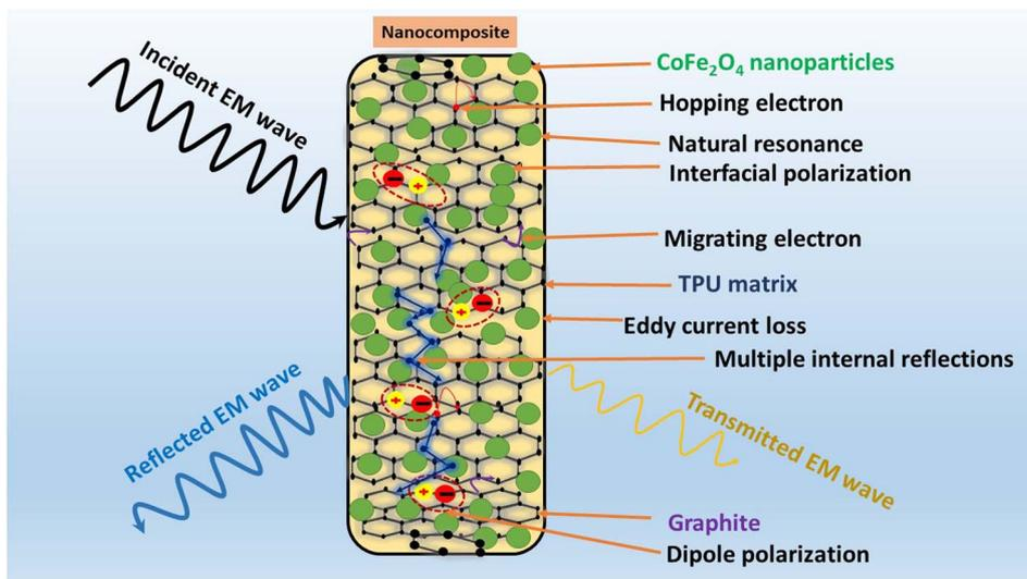
Fig. 12 A putative EMI shielding mechanism behind the superior EMI performance of the developed CoFe<sub>2</sub>O<sub>4</sub> nanoparticles–graphite–TPU nanocomposite.
