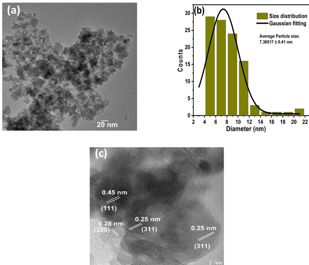
Fig. 3 (a) TEM of the  $\text{CoFe}_2\text{O}_4$  nanoparticles, (b) particle size distribution for  $\text{CoFe}_2\text{O}_4$  nanoparticles, and (c) HRTEM of the  $\text{CoFe}_2\text{O}_4$  nanoparticles.
