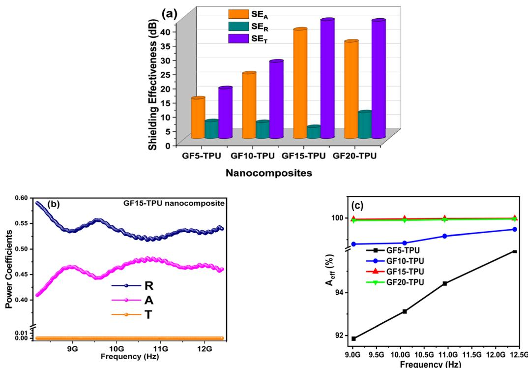
Fig. 7 (a) The comparison plot of the contribution of  $SE_A$ ,  $SE_R$  and  $SE_T$  for the developed GF-TPU nanocomposites, (b) power coefficients for the GF15-TPU nanocomposite, and (c)  $A_{\text{eff}}$  of the developed GF-TPU nanocomposites as a function of frequency.
