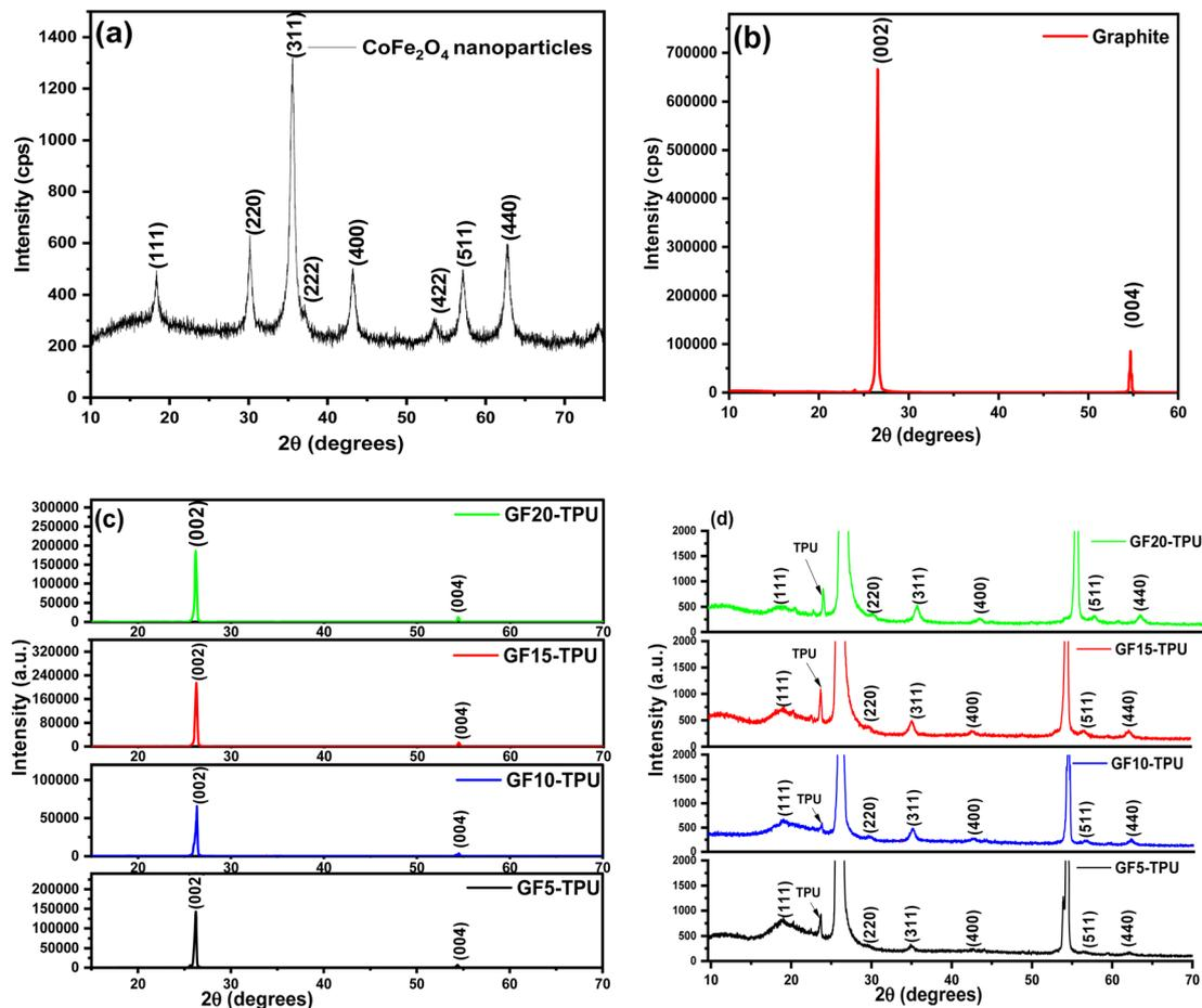
Fig. 2 XRD pattern of (a)  $\text{CoFe}_2\text{O}_4$  nanoparticles, (b) graphite, (c) all the developed GF-TPU nanocomposites; and (d) magnified XRD pattern of all the developed GF-TPU nanocomposites.
