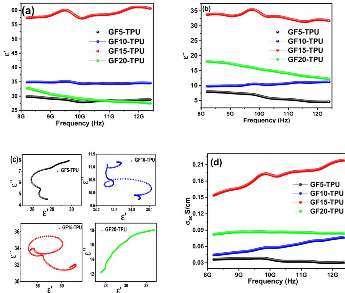
Fig. 9 (a) The real part of the permittivity  $\epsilon'$ , (b) imaginary part of permittivity  $\epsilon''$  as a function of the frequency, (c) Cole–Cole plot, and (d) a.c. conductivity  $\sigma_{ac}$  as a function of frequency for all the developed GF–TPU nanocomposites.
