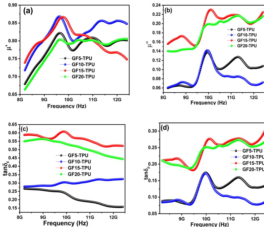
Fig. 10 (a) The real part of the permeability  $\mu'$ , (b) the imaginary part of permeability  $\mu''$ , (c) dielectric loss,  $\tan \delta_e$ , and (d) magnetic loss,  $\tan \delta_\mu$ , as a function of the frequency for all the developed GF-TPU nanocomposites.
