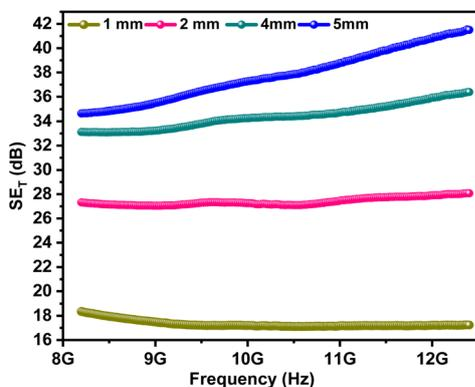
Fig. 8 The variation of SE<sub>T</sub> with tuned thickness as a function of frequency for the developed GF15-TPU nanocomposites.
