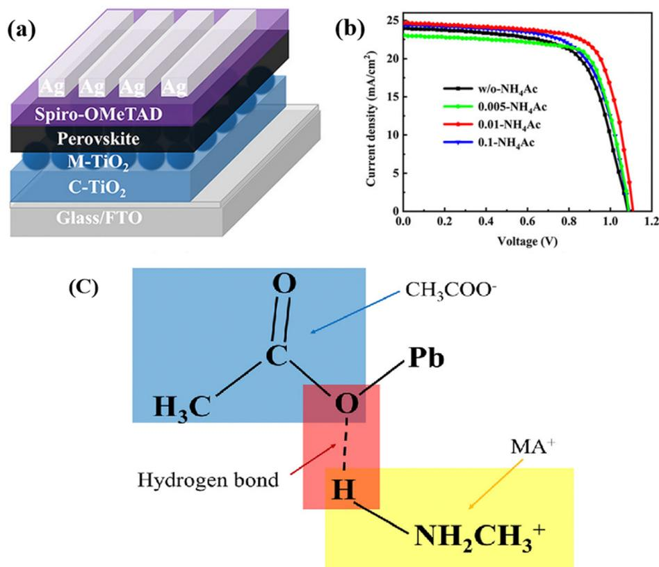
Fig. 3 (a) Architecture of device. (b) *J*-*V* curves of champion devices under different additive concentrations. (c) Schematic diagram of the hydrogen bonding formed between CH<sub>3</sub>COO<sup>-</sup> and MA<sup>+</sup>. Reproduced with permission.<sup>86</sup> Copyright 2021 American Chemical Society.
