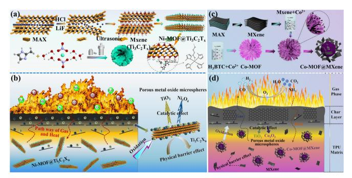
Fig. 6 (a) Schematic synthesis route of Ni-MOF@Ti<sub>3</sub>C<sub>2</sub>T<sub>x</sub> hybrids; (b) flame retardant mechanism of TPU composites. Reproduced with permission from ref. 71, copyright reserved Elsevier 2022. (c) Schematic synthesis route of Co-MOF@MXene hybrids. (d) Flame retardant mechanism of TPU composites. Reproduced with permission from ref. 72, copyright reserved Elsevier 2022.
