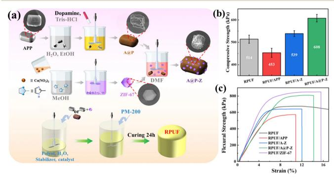
Fig. 9 (a) Flow chart for the preparation of A@P-Z and RPUF composites; (b) 10% compressive strength and (c) flexural strength of RPUF and its composites. Reproduced with permission from ref. 86, copyright reserved Wiley 2018.
