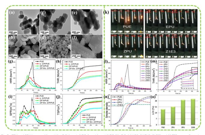
Fig. 3 TEM and SEM images of (a and b)  $\alpha$ -ZrP, (c and d) ZIF-8, and (e and f) ZIF-8/ $\alpha$ -ZrP; (g) HRR, (h) THR, (i) SPR and (j) TSP curves. Reproduced with permission from ref. 46, copyright reserved Wiley 2018. (k) UL-94 vertical burning test; (l) HRR, (m) THR, (n) smoke density, and (o) LOI curves for pure PUE and PUE composites ( $Z_xE_y$  denotes the ZIF-8 to EG ratio of x: y). Reproduced with permission from ref. 47, copyright reserved Wiley 2019.
