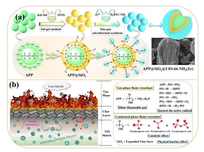
Fig. 5 (a) Schematic of the production route of APP@SiO2@UiO-66-NH2(Zr). (b) Flame retardant mechanism of the TPU composites. Reproduced with permission from ref. 64, copyright reserved Elsevier 2023.
