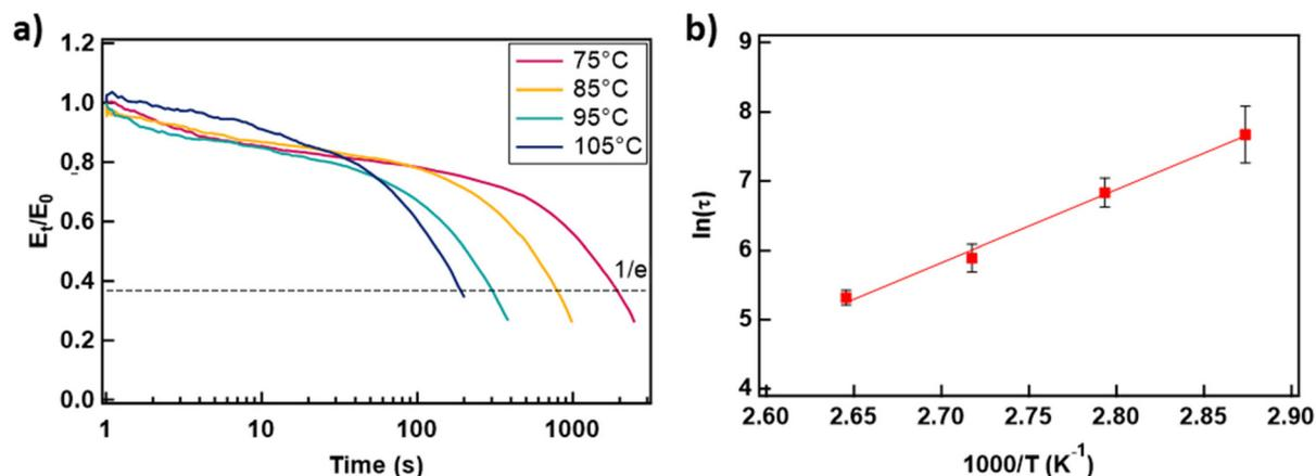
**Fig. 3** (a) Stress relaxation of 7.5–7.5-BVIM gels at varying temperatures. Relaxation times ( $\tau$ ) are determined when the normalized modulus reaches  $1/e$  of the initial value. (b) Activation energy ( $E_a$ ) of Diels–Alder bonds in the network was determined from the slope of the natural logarithm of  $\tau$  plotted against  $1000/T$  ( $E_a = 84 \pm 5 \text{ kJ mol}^{-1}$ ).
