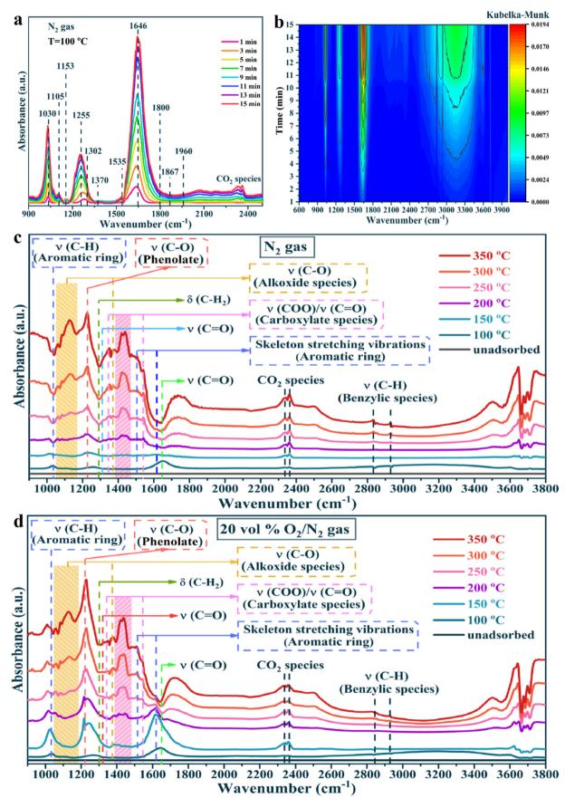
Fig. 9 In situ DRIFTS spectra of toluene adsorption (a and b) for  $Pt_{NC}$ @CeO<sub>2</sub> catalyst at 100 °C for different times under pure  $N_2$  gas flow and the in situ DRIFTS spectra of  $Pt_{NC}$ @CeO<sub>2</sub> catalyst for different reaction temperatures with toluene/ $N_2$  gas (c) and toluene/air gas (d).
