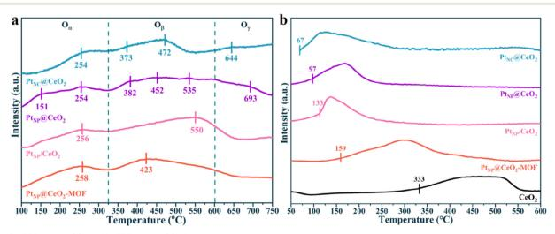
Fig. 7 O<sub>2</sub>-TPD curves (a) and H<sub>2</sub>-TPR curves (b) of samples.
