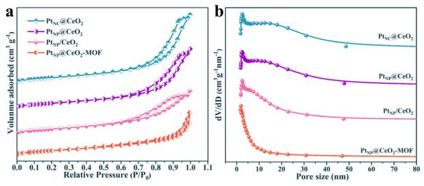
Fig. 5 The N<sub>2</sub> physisorption isotherms of catalysts (a) and the BJH pore size distributions of catalysts (b).
