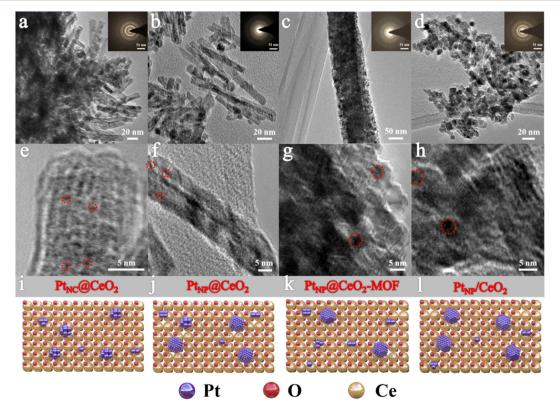
Fig. 2 The TEM images of Pt<sub>NC</sub>@CeO<sub>2</sub> (a and e), Pt<sub>NP</sub>@CeO<sub>2</sub> (b and f), Pt<sub>NP</sub>@CeO<sub>2</sub>-MOF (c and g) and Pt<sub>NP</sub>/CeO<sub>2</sub> (d and h) and the schematic structure of each catalyst (i-I). The inset shows the lattice diffraction rings of each catalyst.
