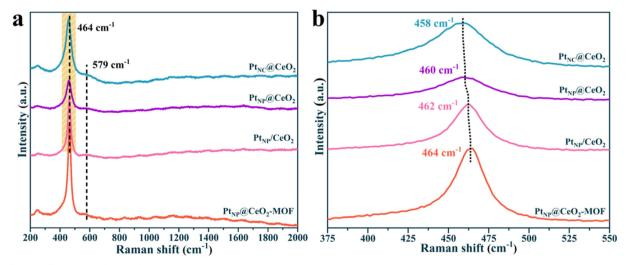
Fig. 4 Raman diagrams of the catalysts
