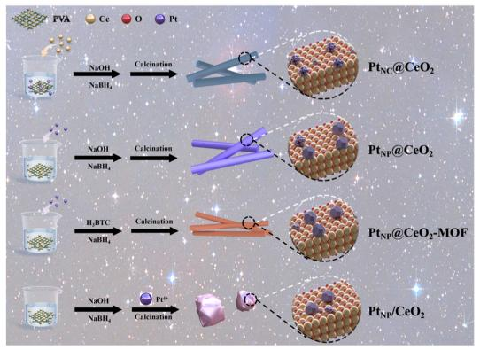
Scheme 1 Schematic illustration of the synthetic process of Pt-CeO<sub>2</sub> catalysts.
