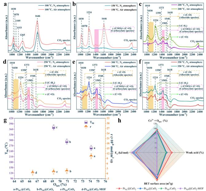
Fig. 10 In situ DRIFTS spectra under different atmospheres at different temperatures (a-f), the reaction rate and  $T_{90}$  versus  $O_{latt}$  (g), and the schematic diagram of  $E_a$  and frame of active sites over the catalysts (h).
