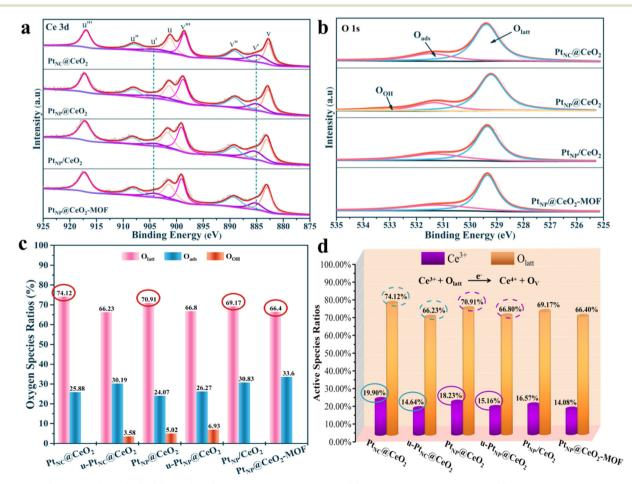
Fig. 6 The XPS spectra about Ce 3d (a) and O 1s (b), the oxygen species ratios (c) and the active species ratios (d) of catalysts.
