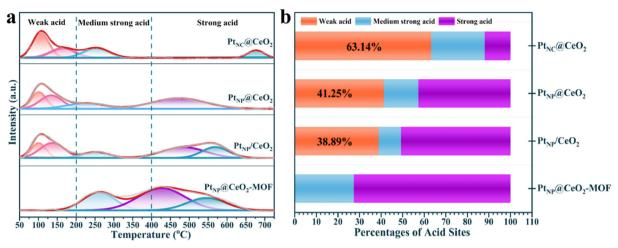
Fig. 8 NH<sub>3</sub>-TPD profiles (a) and percentages of surface acid sites (b) of catalysts.
