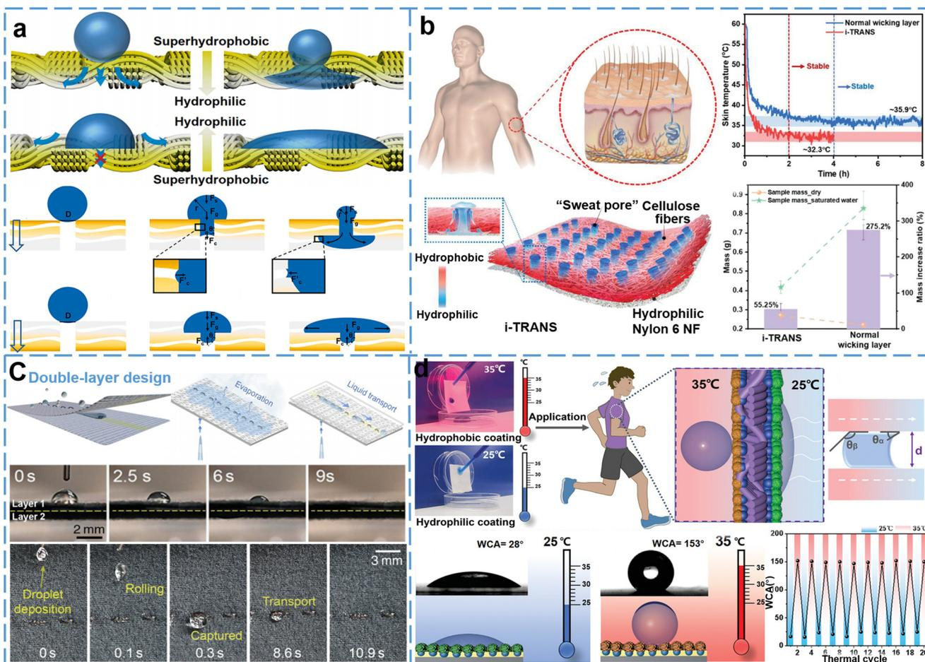
Fig. 9 (a) Janus fabric one-way water transport mechanism,<sup>127</sup> Copyright 2021 Elsevier; (b) concept illustration of integrated 3D hydrophilicity/hydrophobicity design for artificial sweating skin (i-TRANS),<sup>169</sup> Copyright 2022 Wiley-VCH; (c) schematic of the fabrication of the double-layer fabric assembly,<sup>170</sup> Copyright 2023 The Royal Society of Chemistry; (d) temperature triggered directional water transport fabric,<sup>171</sup> Copyright 2023 Wiley-VCH.
