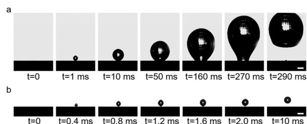
**Fig. 3** Processes of bubble formation in the (a) adsorption state and (b) desorption state in 1 mmol L<sup>-1</sup> SDS solution. Scale, 500 μm.
