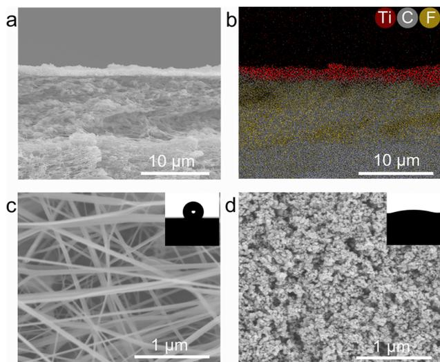
**Fig. 2** Structural characterization of the Rh/TiO<sub>2</sub>-GDL. (a) Cross-sectional SEM image and (b) corresponding EDS mapping of Rh/TiO<sub>2</sub>-GDL; top-view SEM images of (c) pristine GDL porous substrate and (d) immobilized Rh/TiO<sub>2</sub> photocatalyst layer. Inserts in (c) and (d) show photographs of water droplets on each sample.
