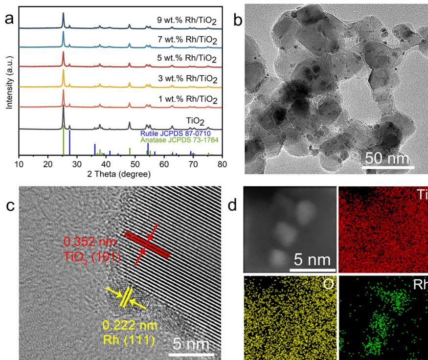
**Fig. 1** Characterization for Rh/TiO<sub>2</sub> photocatalysts. (a) XRD pattern for *x* wt% Rh/TiO<sub>2</sub>; (b) TEM image and (c) high-resolution TEM image of 5 wt% Rh/TiO<sub>2</sub>; (d) the HAADF-STEM image and EDS element maps of 5 wt% Rh/TiO<sub>2</sub>.
