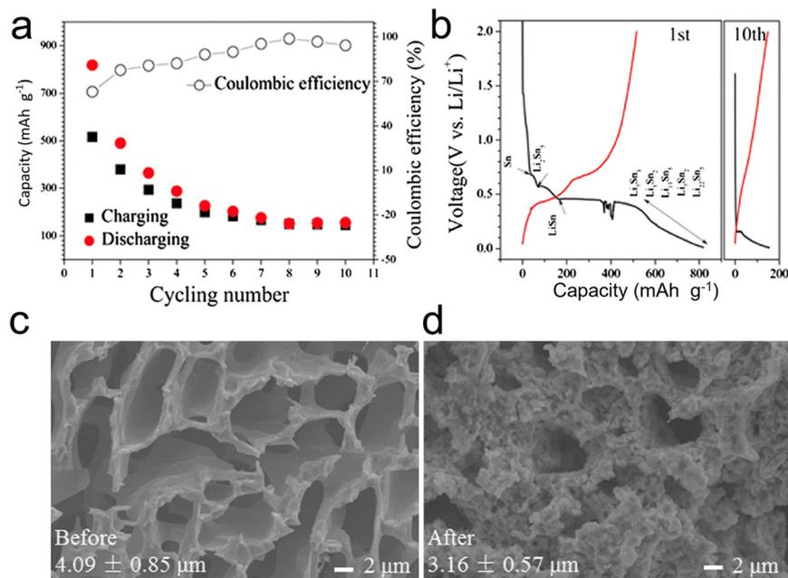
Fig. 14 (a) Cycling performance and (b) charge/discharge curve of the porous Sn dealloyed from  $\text{Al}_{60}\text{Sn}_{20}$ ; SEM images of the porous Sn structure before (c) and after (d) the lithiation/delithiation process. Reprinted with permission from ref. 127. Copyright 2015, Springer.
