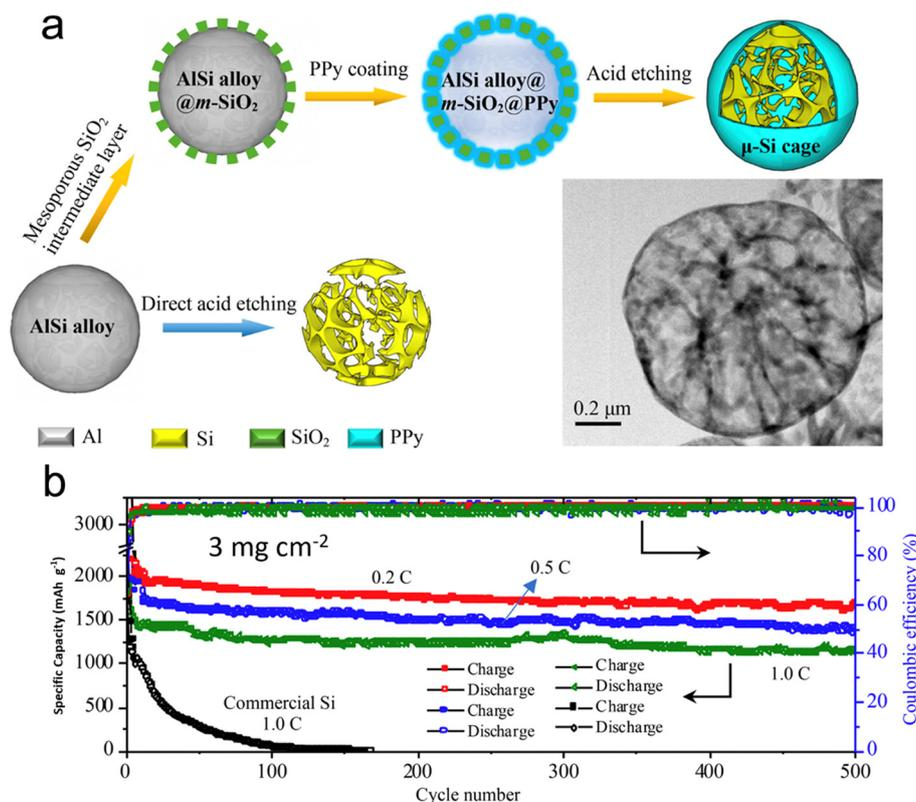
**Fig. 11** (a) Scalable synthesis of the  $\mu$ -Si cage using AlSi microspheres as precursor by a chemical method (inset shows the TEM image of the  $\mu$ -Si cage); (b) cycling performance of the battery with a  $\mu$ -Si cage as anode with loadings of  $3 \text{ mg cm}^{-2}$ . Reprinted with permission from ref. 122. Copyright 2019, American Chemical Society.
