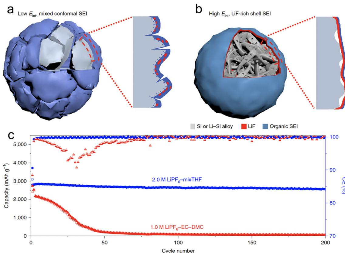
**Fig. 3** Schematic of the cycled alloy anode with an organic, low  $E_{\text{int}}$  and non-uniform (a) and an inorganic, high  $E_{\text{int}}$  and uniform (b) Li alloy-SEI interface; (c) cycling stability and CEs of SiMPs cycled in 2.0 M LiPF<sub>6</sub>-mixTHF and 1.0 M LiPF<sub>6</sub>-EC-DMC electrolytes at C/5. Reprinted with permission from ref. 66. Copyright 2020, Springer Nature.
