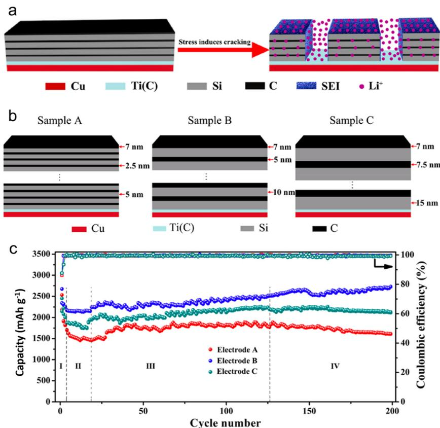
**Fig. 12** (a) Schematic illustration of Si/C multilayer blocks formed by stress; (b) schematic illustration of Si/C multilayer films structure; (c) cycling performance of electrodes A–C at a current density of 300 mA g<sup>-1</sup>. Reprinted with permission from ref. 123. Copyright 2019, American Chemical Society.
