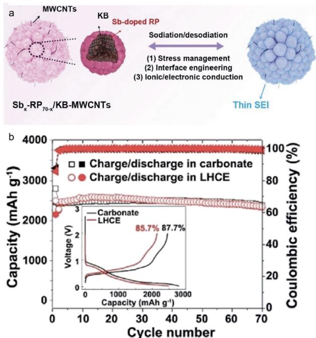
Fig. 13 (a) Schematic illustration and (b) cycling performance in carbonate electrolyte and localized highly concentrated ether electrolyte (LHCE) of hierarchical micro/nanostructured  $\text{Sb}_x\text{-RP}_{70-x}/\text{KB-MWCNTs}$ . Inset: first charge/discharge curve in two electrolytes. Reprinted with permission from ref. 125. Copyright 2021, American Chemical Society.
