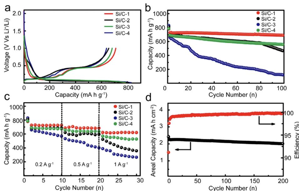
**Fig. 10** (a) The first charge and discharge profiles; (b) the cycling stability; (c) rate capability of different Si/C anodes; (d) high areal mass loading test and coulombic efficiency of the Si/C-1 anode. Reprinted with permission from ref. 117. Copyright 2016, WILEY-VCH Verlag GmbH & Co. KGaA, Weinheim.
