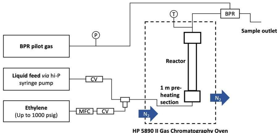
Fig. 2 Flow chemistry setup.
