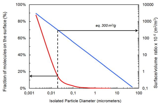
**Fig. 1** Relationship between fraction of molecules on the surface, isolated particle diameter and surface/volume ratio for spheroidal materials, adapted, with permission, from Witschger & Fabriès (2005).<sup>76</sup> Footnotes to figure: the blue line represents the correlation between isolated particles supposed to be spherical and their surface/volume ratio. The red curve represents the correlation between the diameter of these particles and the fraction of atoms at the surface.
