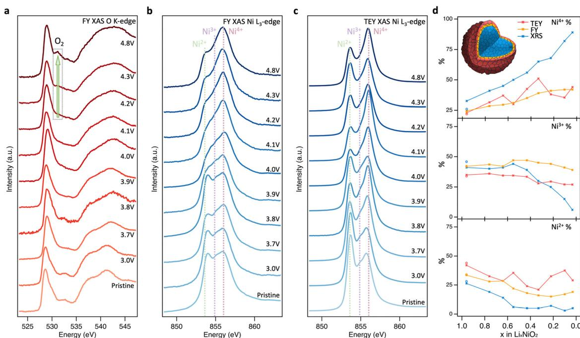
Fig. 2 Near-surface probing of  $\text{LiNiO}_2$  redox processes. (a) and (b) FY-XAS ( $\sim 200$  nm information depth) of the O K-edge and Ni  $L_3$ -edge, and (c) TEY-XAS ( $\sim 10$  nm information depth) of the Ni  $L_3$ -edge for  $\text{LiNiO}_2$  at different SoC. (d) Relative intensities of  $\text{Ni}^{2+}$ ,  $\text{Ni}^{3+}$ , and  $\text{Ni}^{4+}$  components based on fitting CTM calculated spectra to XRS, FY-XAS, and TEY-XAS spectra (see fitting results in ESI† Fig. S2–S5).
