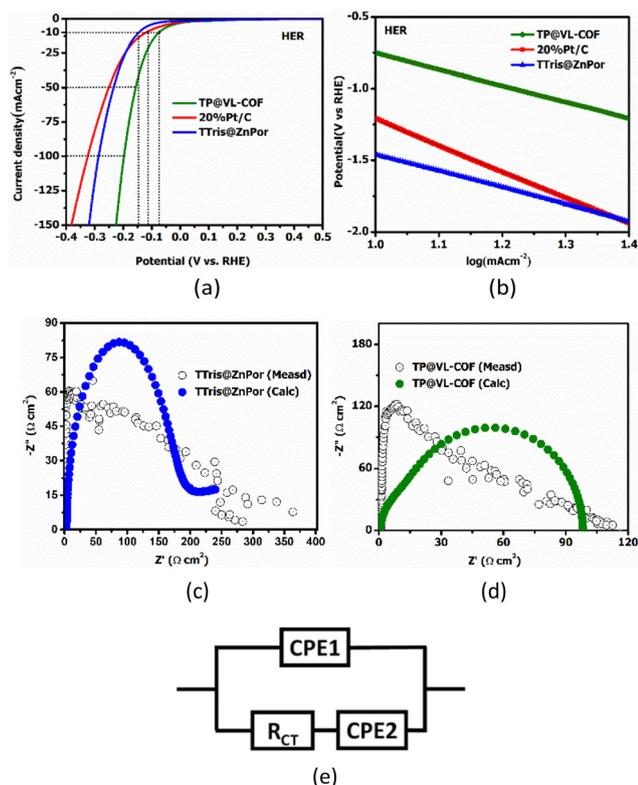
**Fig. 7** Electrocatalysis observations of 20%Pt/C, TTris@ZnPor and TP@VL-COF in an alkaline medium (1 M KOH) at a scan rate of 10 mV s<sup>-1</sup>. (a) LSV curves for the HER. (b) Tafel plots for the HER. Nyquist EIS plots for (c) TTris@ZnPor and (d) TP@VL-COF. (e) EIS equivalent circuit for both TTris@ZnPor and TP@VL-COF.
