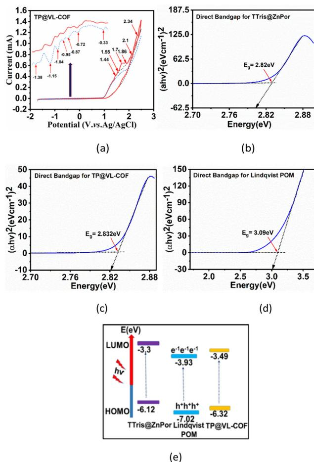
**Fig. 3** (a) Cyclic voltammograms of the TP@VL-COF in DMF/ $CH_3CN$  ( $v/v = 1:1$ ). The supporting electrolyte was TBAP. The zoomed-in portion on the right side of the graph indicates the reduction potential of the TP@VL-COF. The bandgap energy ( $E_g$ ) evaluated through the Tauc plots of (b) TTris@ZnPor, (c) TP@VL-COF and (d) Lindqvist POM. (e) HOMO–LUMO band gaps of TTris@ZnPor, Lindqvist POM and TP@VL-COF.
