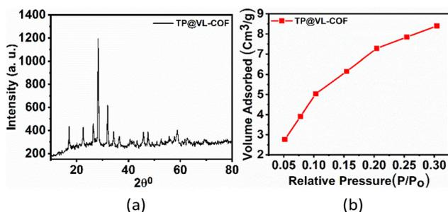
Fig. 5 (a) Powder X-ray diffraction (PXRD) spectrum of the TP@VL-COF. (b) BET N<sub>2</sub>-adsorption isotherm of the TP@VL-COF at 77 K.
