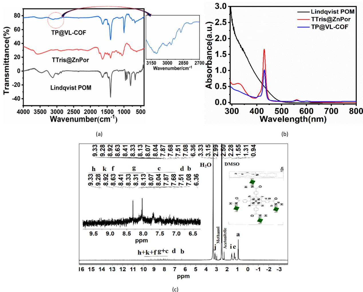
**Fig. 2** (a) Fourier transform infrared spectroscopic (FT-IR) spectra of the TP@VL-COF, TTris@ZnPor and Lindqvist POM. The zoomed-in portion shows the presence of TBA<sup>+</sup> peaks in the TP@VL-COF. (b) UV-vis electronic spectra of TTris@ZnPor, TP@VL-COF and Lindqvist POM. (c) <sup>1</sup>H NMR spectra of the TP@VL-COF.
