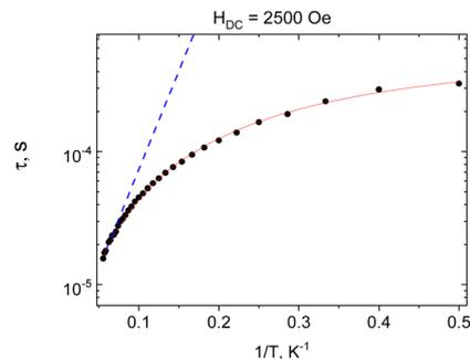
**Fig. 5** Dependence of the relaxation time and the inverse of temperature  $\tau(1/T)$  of **1** ( $H_{\text{DC}} = 2500 \text{ Oe}$ ). Blue dotted line – approximation of the high temperature part by the Arrhenius law. Red solid line – approximation by the sum of Raman and QTM-type contributions. Black circles – experimental data.
