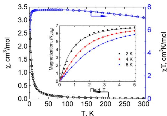
**Fig. 2** Temperature dependence of  $\chi T$  for **1** measured at  $H_{DC} = 5000$  Oe. Inset: magnetization vs. field for **1** measured at  $T = 2, 4$  and  $6$  K. Theoretical curves (solid lines) are calculated with  $J_{Mn1-Mn2} = +67.3(3)$  cm<sup>-1</sup>,  $g_{iso}(Mn1) = 1.960(8)$ ,  $g_{iso}(Mn2) = 1.998(3)$ ,  $D_{Mn2} = -0.727(8)$  cm<sup>-1</sup>,  $zJ' = -0.00321(12)$  cm<sup>-1</sup>.
