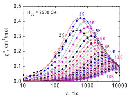
**Fig. 4** Frequency dependence of the imaginary component ( $\chi''$ ) of dynamic magnetic susceptibility for **1** in the range 2–18 K at a dc supporting magnetic field of  $H_{\text{DC}} = 2500 \text{ Oe}$ . Solid lines are approximations of the experimental data using a generalized Debye model.
