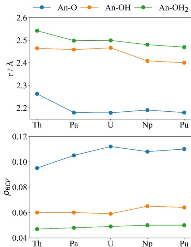
Fig. 7 Optimised distances  $r$  ( $\text{\AA}$ , upper) and  $\rho_{\text{BCP}}$  (a.u., lower) for  $[(\text{An}(\text{H}_2\text{O})_5)(\text{Na}(\text{H}_2\text{O})_2)_5\text{Fe}_{13}\text{O}_{28}\text{H}_{12}]^{4+}$  (calculated at the PBE0/Def2TZVP/SARC-DKH2 level).
