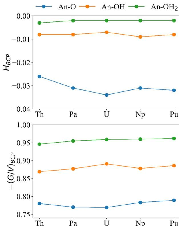
Fig. 8  $H_{\text{BCP}}$  and  $-(G/V)_{\text{BCP}}$  (a.u.) for the An–O, An–OH, and An–OH<sub>2</sub> bonds in  $[(\text{An}(\text{H}_2\text{O})_5)(\text{Na}(\text{H}_2\text{O})_2)_5\text{Fe}_{13}\text{O}_{28}\text{H}_{12}]^{4+}$  (calculated at the PBE0/Def2TZVP/SARC-DKH2 level).
