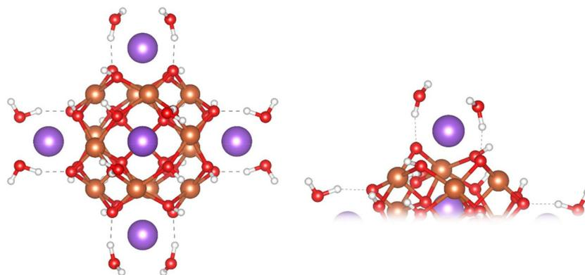
**Fig. 1** Ball and stick images of the optimised geometry of the Na<sup>+</sup>-capped Fe<sub>13</sub> Keggin model (left), close up of the “square-window” (right). Colour scheme: Fe, orange; O, red; H, white; Na, purple.
