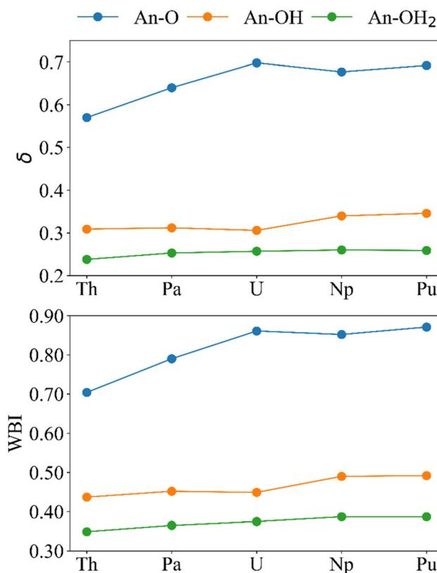
Fig. 6 Bond order metrics for  $[(\text{An}(\text{H}_2\text{O})_5)(\text{Na}(\text{H}_2\text{O})_2)_5\text{Fe}_{13}\text{O}_{28}\text{H}_{12}]^{4+}$ . Upper; delocalisation indices and lower; Wiberg bond indices (calculated at the PBE0/Def2TZVP/SARC-DKH2 level).
