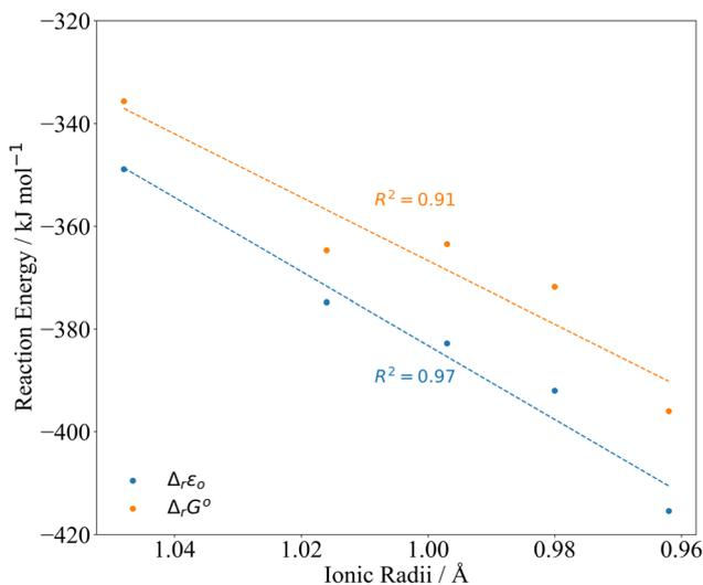
Fig. 4 PBE0/Def2TZVP/SARC-DKH2 reaction energy  $\Delta_r$  according to eqn (2) compared to 8-coordinate An(IV) ionic radii.<sup>45</sup>
