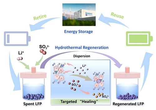
Hydrothermal regeneration of the spent LIBs as a closed-loop recycling. Reproduced with permission from ref. 123; Copyright 2023, Elsevier.
