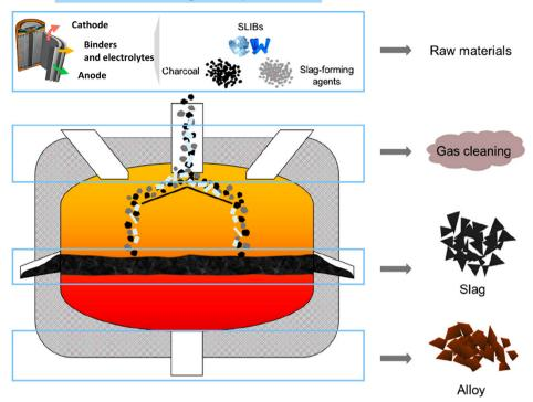
Fig. 4 Typical pyrometallurgical processes of spent LIBs. Reproduced with permission from ref. 62; Copyright 2021, American Chemical Society.
