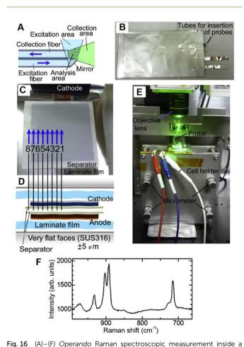
laminate cell using microprobes. (A) Schematic of probe consisting of one excitation optical fiber and one collection fiber. (B) Photograph of a laminate cell inserted with eight microprobes. (C) Inside and (D) cross-section view of the laminate cell with the probes. (E) Photograph of setup of the *operando* fiber-based Raman spectroscopic measurement. (F) Raman spectrum of electrolyte inside the laminate cell. Reproduced with permission from ref. 130. Copyright 2017 Elsevier B.V.
