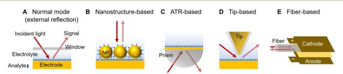
Fig. 4 Different electrochemical vibrational spectroscopic modes. (A) Normal mode (external reflection). (B) Nanostructure-based mode. NP is an abbreviation for nanoparticle. (C) ATR-based mode. (D) Tip-based mode. (E) Fiber-based mode.
