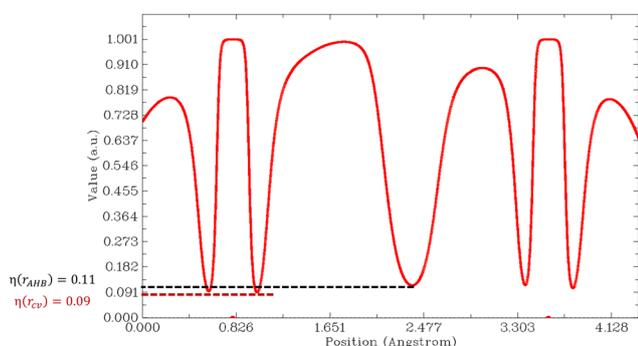
Fig. 6 Variations in the ELF value along the A–H–B bond path for compound DMI\_1. Position  $\eta(r_{\text{cv}})$  corresponds to the lowest value of the ELF for which the core basins are separated from the valence, and  $\eta(r_{\text{AHB}})$  is the value at the saddle point between the  $V(\text{A,H})$  and  $V(\text{B})$  basins.
