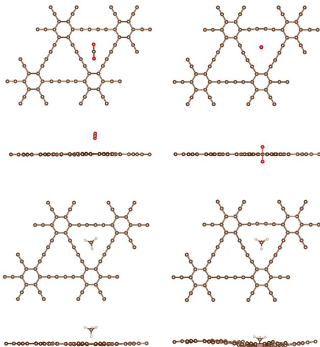
Fig. 5 Top and lateral views of the orientation of the CO<sub>2</sub> molecule on GDY, at  $z = 3 \text{ \AA}$ , and  $z = 0$ . Same for CH<sub>4</sub> at  $z = 2 \text{ \AA}$ , and  $z = 0$ . The calculations assume  $x = y = 0$ . Oxygen, carbon and hydrogen atoms are represented by red, brown, and light grey spheres, respectively.
