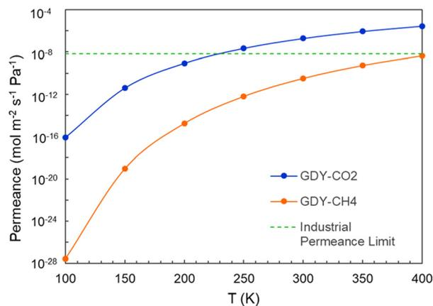
Fig. 13 Permeance of CO<sub>2</sub> and CH<sub>4</sub> through GDY as a function of temperature for an incoming pressure  $p = 3 \times 10^5$  Pa and a pressure difference between the two sides of the membrane  $\Delta p = 10^5$  Pa. The horizontal line represents the industrial permeance limit.
