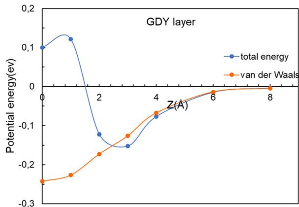
Fig. 7 Energy as a function of the distance  $z$  between the CO<sub>2</sub> molecule and the GDY layer. The  $(x, y)$  coordinates of the molecule are  $x = 0, y = 0$ . The van der Waals contribution is also included.
