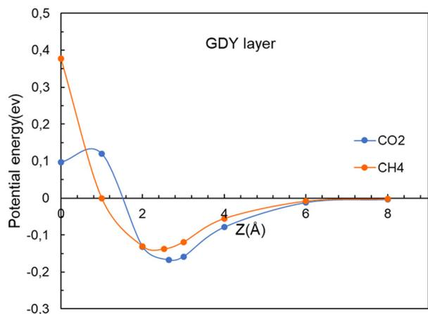
Fig. 8 Energy as a function of the distance  $z$  between the CO<sub>2</sub> and CH<sub>4</sub> molecules and the GDY layer. The  $(x, y)$  coordinates of the molecules are relaxed for each value of  $z$ .
