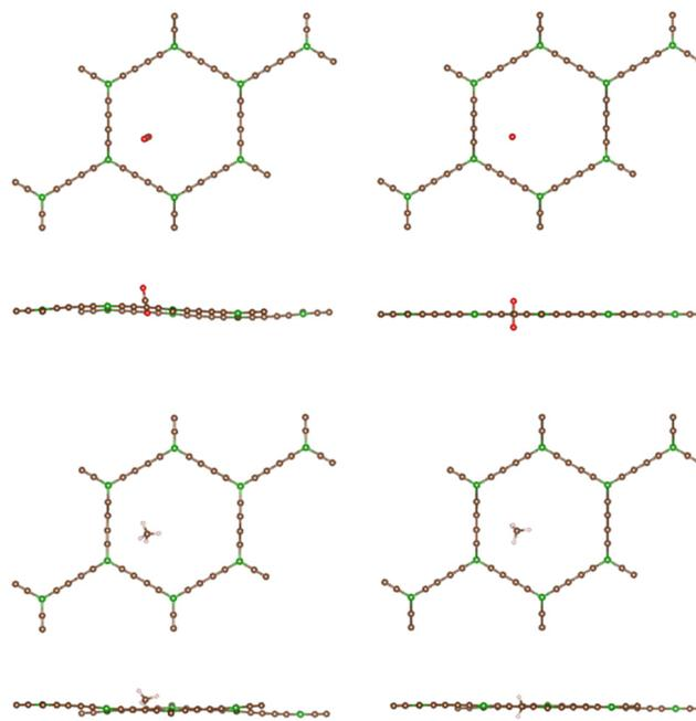
Fig. 10 Top and lateral views of the orientation of the  $\text{CO}_2$  and  $\text{CH}_4$  molecules on BGDY, at  $z = 1 \text{ Å}$ , and  $z = 0$ . Oxygen, carbon and hydrogen atoms are represented by red, brown, and light grey spheres, respectively. The  $(x, y)$  coordinates of the center of mass of the molecules are relaxed for each value of  $z$ .
