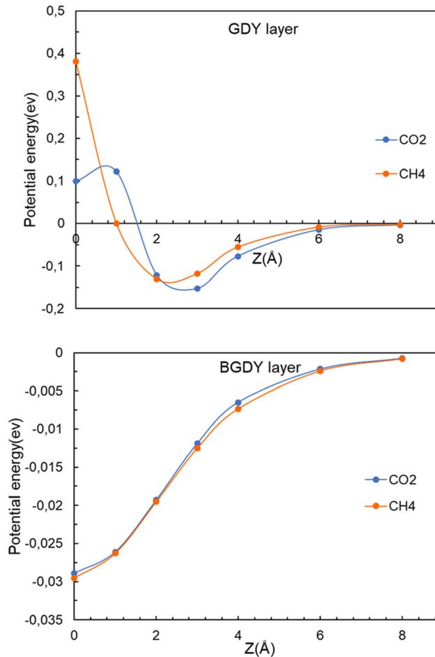
Fig. 4 Energy as a function of the distance  $z$  between the CO<sub>2</sub> or CH<sub>4</sub> molecules and the layer. Upper panel, GDY. Lower panel, BGDY. The  $(x, y)$  coordinates of the molecule are  $x = 0, y = 0$ .
