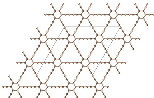
Fig. 1 Planar structure of graphdiyne, showing hexagonal rings linked by diacetylenic  $-\text{C}\equiv\text{C}-\text{C}\equiv\text{C}-$  chains, which form large triangular holes. The unit cell used in the calculations is highlighted.
