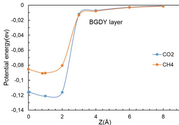
Fig. 9 Energy as a function of the distance  $z$  between the  $\text{CO}_2$  and  $\text{CH}_4$  molecules and the BGDY layer. The  $(x, y)$  coordinates of the molecules are relaxed for each value of the vertical distance  $z$ .
