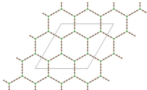
Fig. 2 Planar honeycomb structure of boron graphdiyne, showing hexagonal holes. BGDY is formed by boron atoms connected by carbon chains containing diacetylenic  $-\text{C}\equiv\text{C}-\text{C}\equiv\text{C}-$  linkages. Boron and carbon atoms are represented by green and brown spheres, respectively. The unit cell used in the calculations is highlighted.
