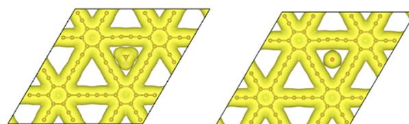
Fig. 11 Top view of the electronic density of  $\text{CH}_4$  (left panel) and  $\text{CO}_2$  (right panel) at the point of passing through the GDY membrane,  $z = 0$ . The yellow regions correspond to a surface of constant electron density with the value  $0.01 \text{ e a.u.}^{-3}$ .
