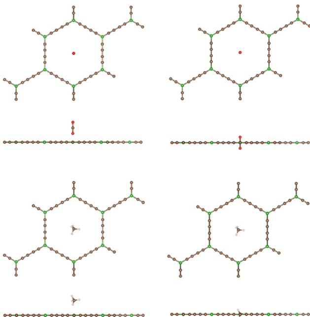
Fig. 6 Top and lateral views of the orientation of the CO<sub>2</sub> molecule at  $z = 3 \text{ \AA}$ , and on the plane of the BGDY layer,  $z = 0 \text{ \AA}$ . Same for CH<sub>4</sub>. The calculations assume  $x = y = 0$ . Oxygen, carbon and hydrogen atoms are represented by red, brown, and light grey spheres, respectively.
