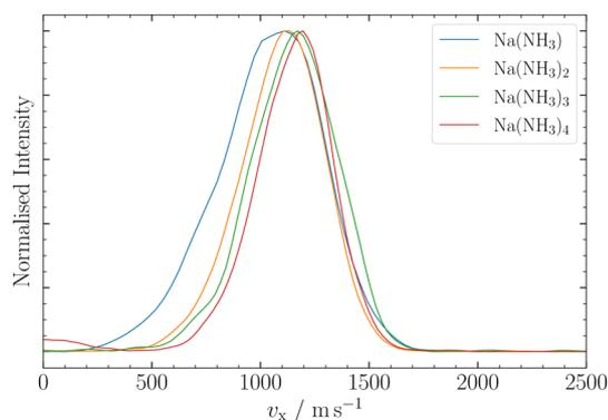
Fig. 5 Ion VMI results for  $\text{Na}(\text{NH}_3)_n$ ,  $n = 1-4$ .  $\text{Na}(\text{NH}_3)_1$  and  $\text{Na}(\text{NH}_3)_2$  were measured with a nozzle temperature of  $T = 25 \text{ }^\circ\text{C}$ , whereas  $\text{Na}(\text{NH}_3)_3$  and  $\text{Na}(\text{NH}_3)_4$  were measured at  $T = 100 \text{ }^\circ\text{C}$ .
