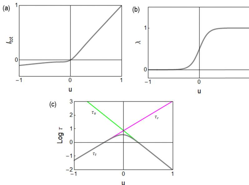
Fig. 4 (a) Current–voltage curve. (b) Equilibrium value of the state variable. (c) Relaxation times. Parameters  $V_s = 0.3$ ,  $V_r = -0.4$ ,  $V_m = 0.1$ ,  $n_s = 1.5$ ,  $n_r = 2$ ,  $g_L = 0.1$ ,  $g_H = 1$ , and  $\tau_k = 1$ .
