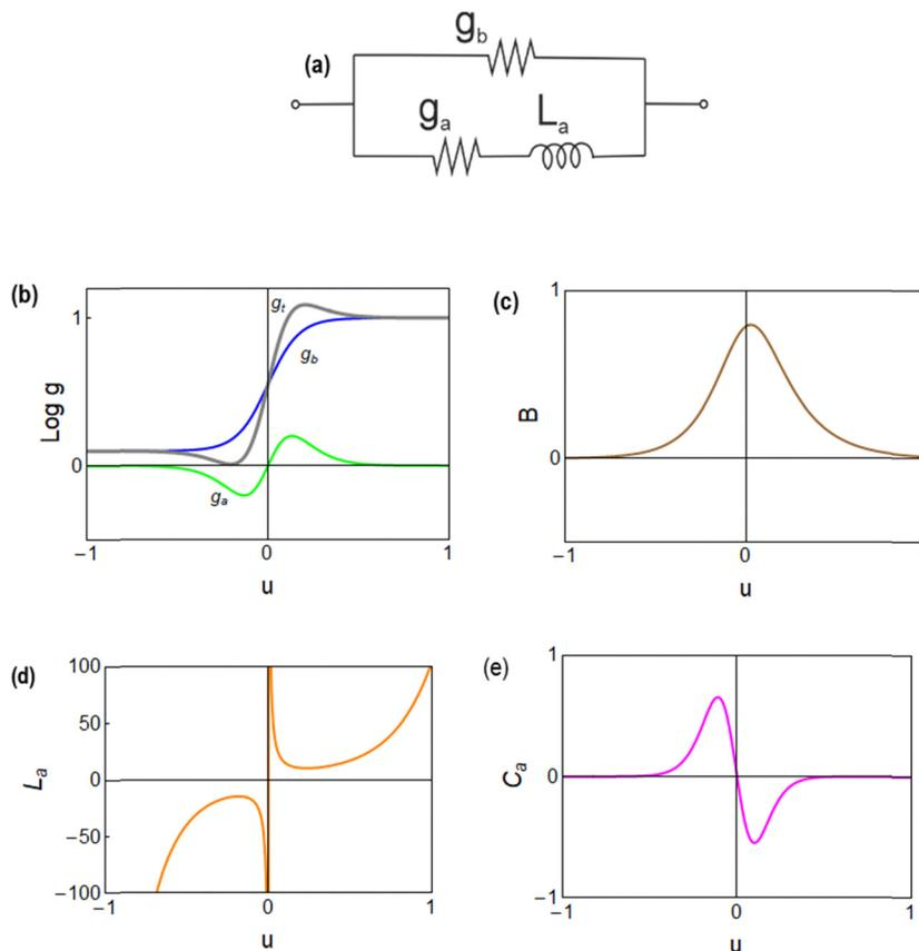
Fig. 6 (a) Equivalent circuit. Functions determining the impedance response. (b) Differential conductances,  $g_t = g_b + g_a$ . (c)  $B$ . (d) Inductor. (e) Effective low frequency capacitance. Parameters as in Fig. 4.
