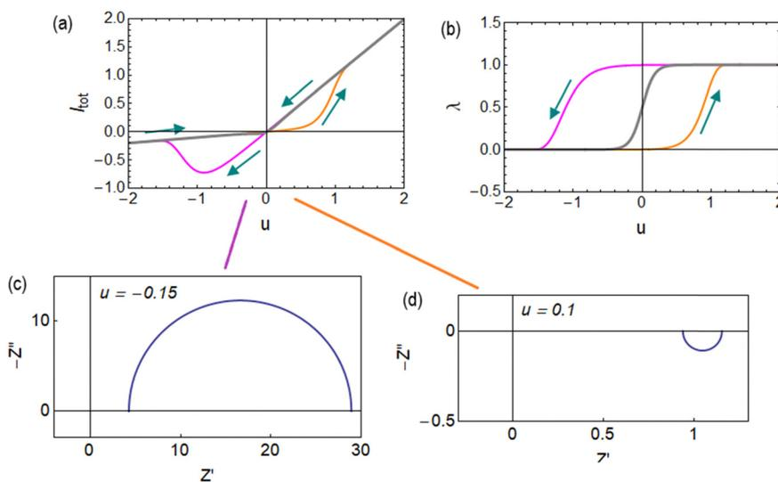
Fig. 5 Hysteresis at a rate  $v_{\text{scan}} = 10$  in (a) current–voltage curves and (b) state variable. The grey lines are the equilibrium curves. (c) and (d) Impedance spectra at the indicated voltage points. Parameters as in Fig. 4.
