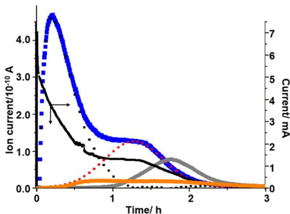
Fig. 6 Time dependencies of current (black) and signals of  $m/z = 18$  (orange), 32 (blue), and 44 (gray) when the voltage was stepped from 2.8 V to 4.4 V. The red dotted line shows Gaussian fitting for the 2nd oxygen generation and the black dotted line is the residue for  $O_2$  generation after the subtraction of the red curve.
