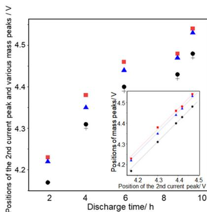
Fig. 9 Positions of the second peak of current (+), 18 ( $\blacksquare$ ), and 32 ( $\bullet$ ), and the peak of 44 ( $\blacktriangle$ ) as a function of discharge time. Inset: Positions of the second peak of 18 ( $\blacksquare$ ) and 32 ( $\bullet$ ), and the peak of 44 ( $\blacktriangle$ ) as a function of the positions of the second current peak.
