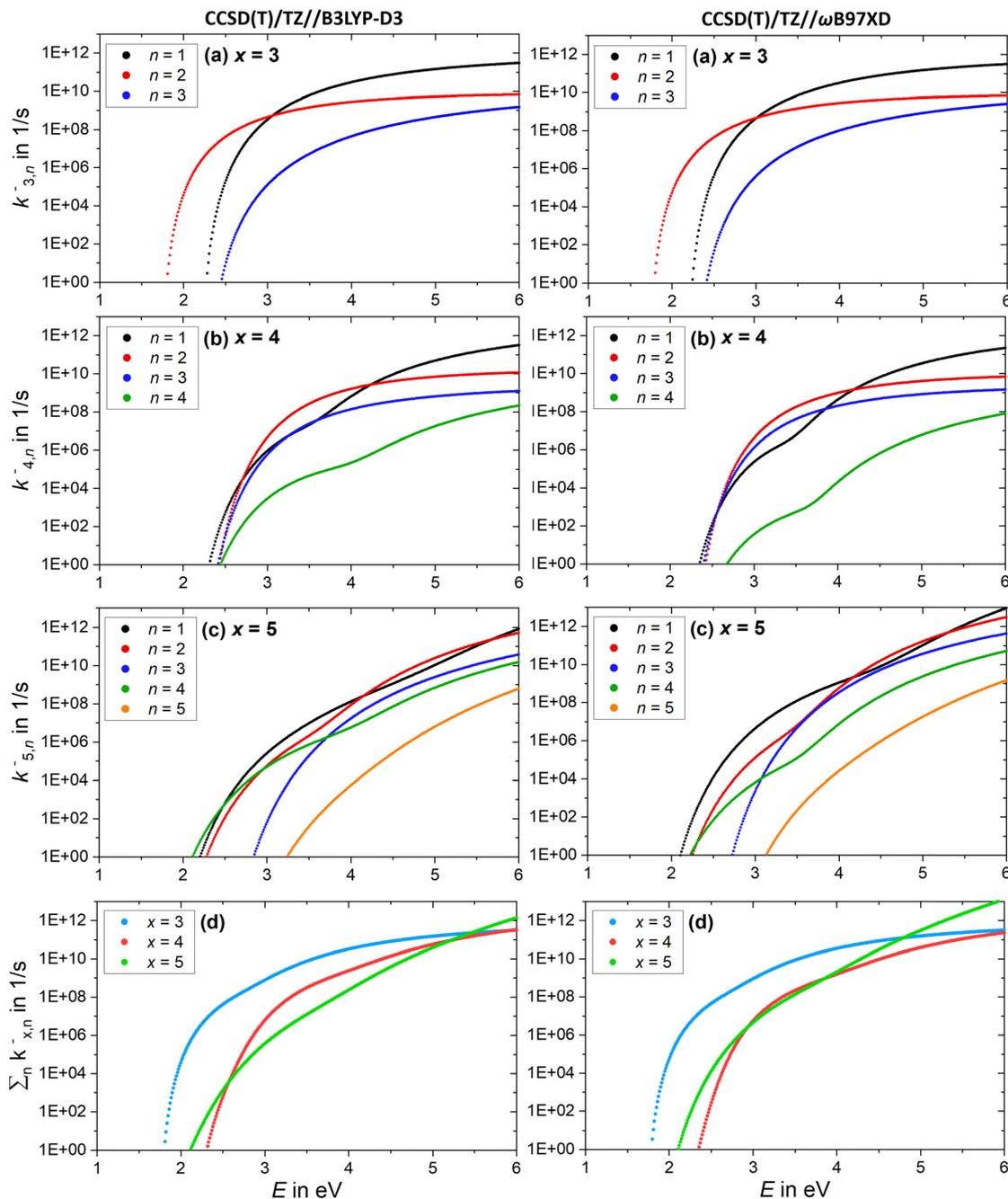
Fig. 9 (a)–(c) Calculated RRKM rate constants  $k_{x,n}^-$  for the loss channels (3) of the precursor ions  $(\text{NaCl})_x\text{Cl}^-$  with  $x = 3$ –5. Note that the loss channels producing  $\text{Cl}^-$  ions ( $k_{x,n=x}^-$ ) are always the slowest. (d) Total fragmentation rate constants  $\sum_n k_{x,n}^-$  as sum of all loss channels  $n$  for cluster sizes  $x = 3$ –5.
