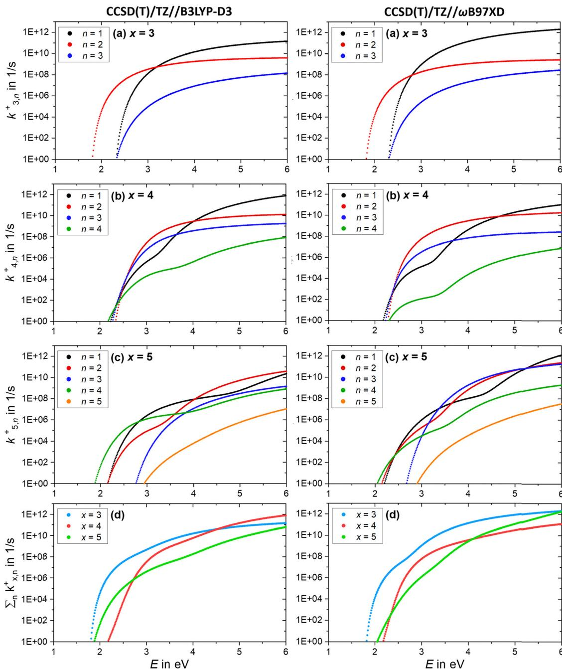
**Fig. 8** (a)–(c) Calculated RRKM rate constants  $k_{x,n}^+$  for the loss channels (2) of the precursor ions  $(\text{NaCl})_x\text{Na}^+$  with  $x = 3$ –5. Note that the loss channels producing  $\text{Na}^+$  ions ( $k_{x,n=x}^+$ ), which cannot be detected in the experiment, are always the slowest at higher energies. (d) Total fragmentation rate constants  $\sum_n k_{x,n}^+$  as sum of all loss channels  $n$  for cluster sizes  $x = 3$ –5.
