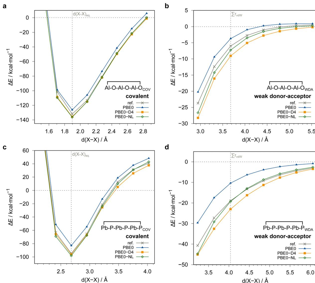
Fig. 10 Rigid potential energy scans of the covalent and weak donor-acceptor dimers with respect to the planar monomer fragments.  $d(X-X)$  is the center-of-ring-atoms inter-fragment distance. The grey reference curve was obtained with PNO-LCCSD(T)-F12/awcvtz with PROJECTOR=MIXED and TRHPNO\_LMP2=1d-10. All energies in  $\text{kcal mol}^{-1}$ .
