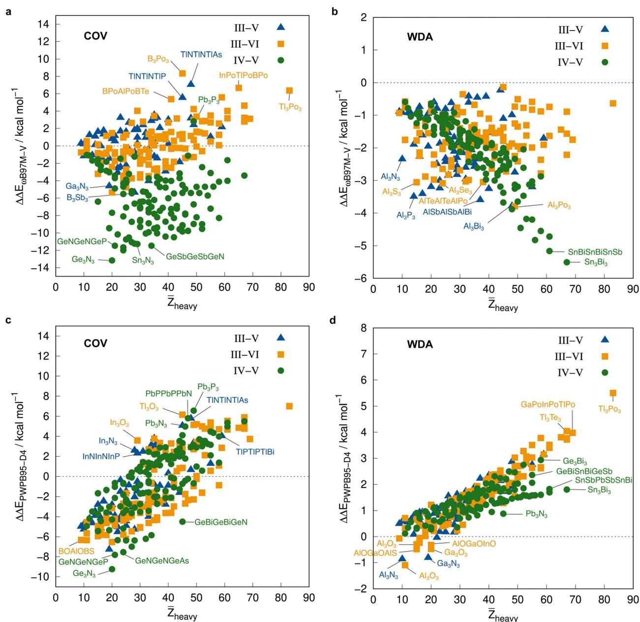
Fig. 11 Correlation plot of the DFT dimerization energies in  $\text{kcal mol}^{-1}$  and the mean atomic number of the involved heavy atoms for covalent and weak donor-acceptor bound systems computed with  $\omega\text{B97M-V}$  (a) and (b), and PWPB95-D4 (c) and (d), respectively.
