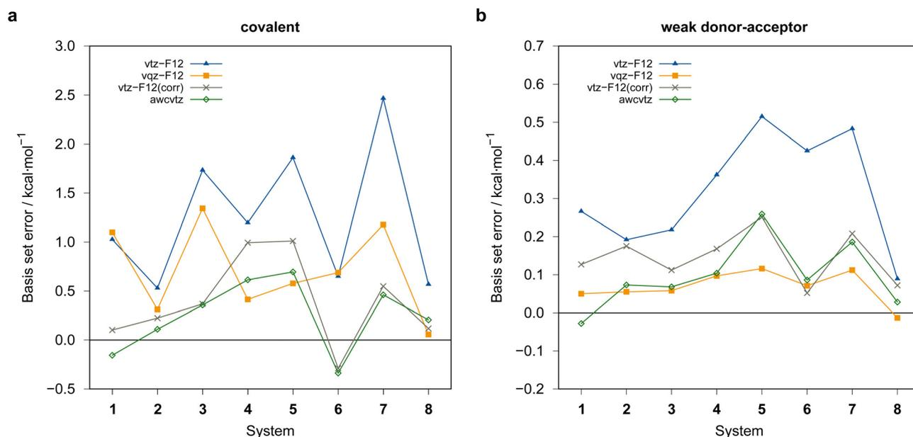
Fig. 6 PNO-LCCSD(T)-F12 basis set errors (in  $\text{kcal mol}^{-1}$ ) relative to the PNO-LCCSD(T)-F12/awcvtz reference values (using PROJECTOR=MIXED and THRPNO\_LMP2=1d-10 except for vtz-f12(corr.), see text). (a) Covalent dimers, (b) weak donor-acceptor dimers. vqz-f12 values computed with  $\gamma$  (opt3), otherwise  $\gamma = [1.0, 1.4]$  was employed.
