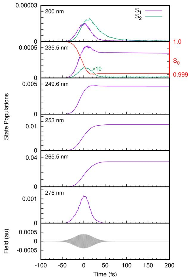
Fig. 6 The time evolution of the  $S_1$  and  $S_2$  state populations following excitation from the  $S_0$  state for different wavelengths. The electric field corresponding to a 235.5 nm pulse is also plotted as a guide to the eye. The depletion of the  $S_0$  state population (scale on the right-hand axis) for the 235.5 nm pulse indicates a shoulder region (ca. 30 fs) similar to  $S_1$ . The  $S_2$  population for the 235.5 nm pulse is multiplied by a factor of 10 for better visualization.
