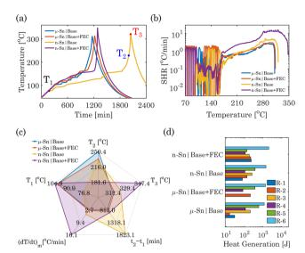
Fig. 2 The ARC experiments to probe the thermal stability of the Sn electrode. (a) Temperature response of  $\mu\text{-Sn}$  and n-Sn-based half-cell using the electrolytes-base and base + FEC. (b) The temperature increase and the corresponding self-heating rates (SHR) for all the cases. (c) Thermal safety characteristics and (d) comparison of heat generation of the  $\mu$  and n-Sn cases in two different electrolytes.
