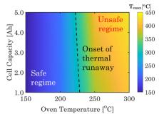
Fig. 4 Thermal safety phase map for the NVP-μ-Sn-based SIBS under different capacity and oven temperatures. The black line represents the initiation of thermal runaway under oven conditions.
