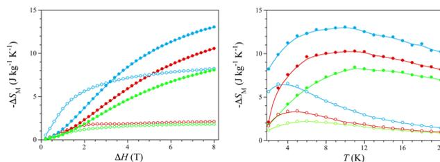
Fig. 3 Isothermal (left) and isofield (right) curves of the magnetic entropy change for **1** (red), **2** (green), and **3** (blue) at 2 (○)/10 K (●) and 2 (○)/8 T (●), respectively. The solid lines are only eye-guides.
