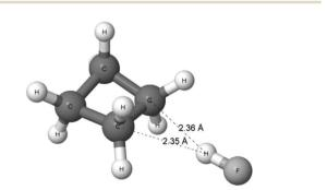
Fig. 9 The complex of cyclobutane with hydrogen fluoride. The H···C distances are indicated.
