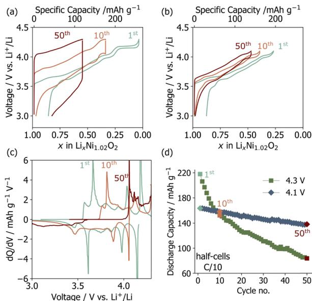
**Fig. 1** Electrochemical data for  $\text{LiNiO}_2/\text{Li}$  half cells cycled at a rate of C/10 ( $C = 200 \text{ mA g}^{-1}$ ). Voltage profiles for selected cycles are shown for the (a) 4.3 V and (b) 4.1 V upper cut-off voltage. (c) Differential capacity,  $dQ/dV$  ( $\text{mA h g}^{-1} \text{ V}^{-1}$ ), plot for a cell cycled to 4.3 V. (d) The average discharge capacity of three cells cycled up to 4.3 V or 4.1 V over 50 cycles.
