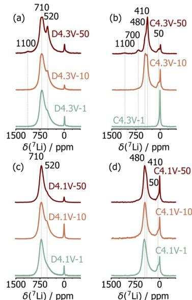
Fig. 3  $^7\text{Li}$  solid-state NMR spectra collected on *ex situ* samples in the (a) and (c) discharged and (b) and (d) charged states for cells cycled to (a) and (b) 4.3 V and (c) and (d) 4.1 V. All spectra were acquired at 2.35 T and 60 kHz MAS and are normalized to the most intense signal.
