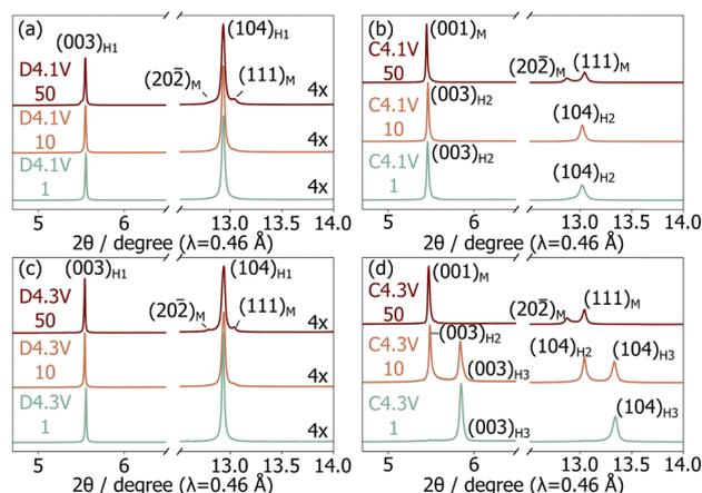
**Fig. 2** Selected regions from the synchrotron XRD patterns collected on *ex situ* samples in the (a) and (c) discharged and (b) and (d) charged states for cells cycled up to (a) and (b) 4.1 V and (c) and (d) 4.3 V. Crystallographic parameters derived from the refinements are tabulated in Table S1 (ESI†) and full synchrotron XRD patterns are provided in Fig. S3–S6 (ESI†).
