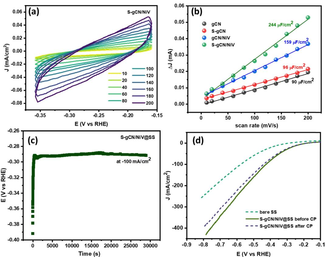
Fig. 7 (a) CV curves measured at different scan rates in the non-faradaic region for S-gCN/NiV. (b) Plot of the double layer charging current density vs. scan rate to illustrate  $C_{dl}$ . (c) Chronopotentiometric analysis of S-gCN/NiV coated on SS at  $-100 \text{ mA}/\text{cm}^2$  for  $\sim 8 \text{ h}$ . (d) LSV curves of S-gCN/NiV@SS recorded before and after chronopotentiometry; the curve of bare SS is shown for comparison.
