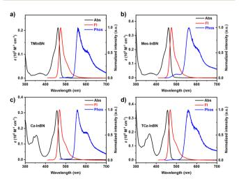
Fig. 3 UV-vis absorption (black line), normalized fluorescence (red line,  $\lambda_{\text{ex}}$ : 400 nm), and phosphorescence (blue line,  $\lambda_{\text{ex}}$ : 420 nm, delay: 25 ms) spectra of (a) TMInBN, (b) Mes-InBN, (c) Cz-InBN, and (d) TCz-InBN in toluene solution (1  $\times$  10<sup>-5</sup> M)
