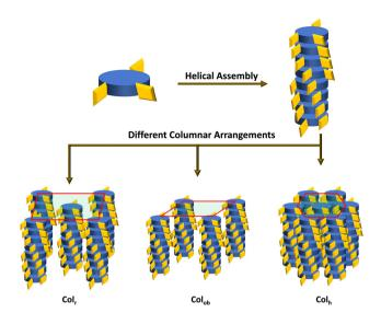
Schematic representation of helicoidal columns arranged in different columnar organization modes.
