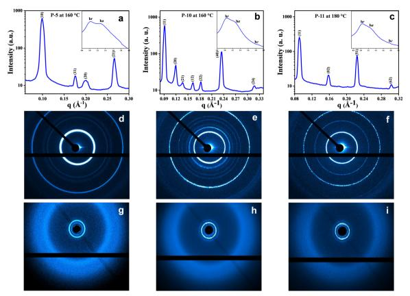
Fig. 4 Small- and wide-angle (inset) X-ray diffraction patterns of the Col phases formed by compounds (a) P-5 at 160 °C (Col<sub>n</sub>), (b) P-10 at 160 °C (Col<sub>ob</sub>) and (c) P-11 at 180 °C (Col<sub>r</sub>) upon cooling (h<sub>r</sub>, cholesterol-cholesterol correlation; h<sub>a</sub>, alkyl chain-chain correlation; h<sub>c</sub>, disc-disc correlation). The lower panels show the respective 2D SAXS (d-f) and WAXS (g-i) diffraction patterns for the compounds in (a-c).
