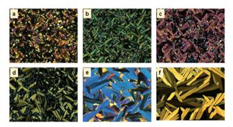
Fig. 3 POM microphotographs of the optical texture of Col phases formed by (a) **P-5** at 280  $^{\circ}$ C, (b) **P-6** at 230  $^{\circ}$ C, (c) **P-7** at 225  $^{\circ}$ C, (d) **P-8** at 190.7 °C, (e) **P-10** at 150.9 °C and (f) **P-11** at 214.9 °C.
