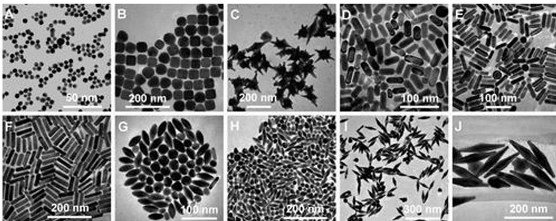
**Fig. 1** Tem images of AuNPs of different shapes and sizes. (A) Nanospheres. (B) Nanocubes. (C) Nanobranches. (D) Nanorods. (E) Nanorods. (F) Nanorods. (G) Nanobipyramids. (H) Nanobipyramids. (I) Nanobipyramids. (J) Nanobipyramids. Reprinted with permission from ref. 27. Copyright © 2008, American Chemical Society.
