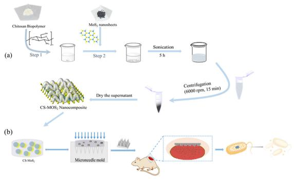
Fig. 1 The synthesis process of the CS-MoS<sub>2</sub> nanocomposite (a); the preparation process and the schematic diagram of the effect of CS-MoS<sub>2</sub> MN on the wound (b)
