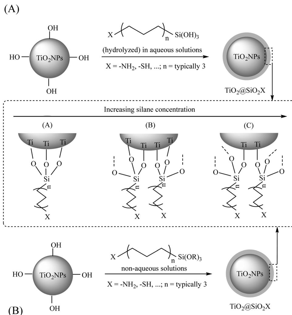
Fig. 3 The interaction between a general silane coupling agent and TiO<sub>2</sub>NPs in aqueous (A) and non-aqueous (B) solutions. Adapted with permission from ref. 22. Royal Society of Chemistry.
