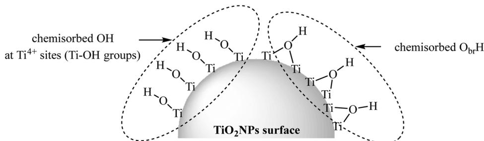
Fig. 1 Two different OH groups of the  $\text{TiO}_2\text{NP}$  surface. Adapted with permission from ref. 20. Copyright 2014 American Chemical Society.
