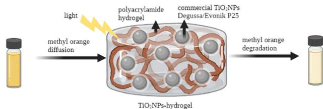
Fig. 4 TiO<sub>2</sub>NP–hydrogel system for the photocatalytic degradation of methyl orange. Adapted with permission from ref. 139. Copyright 2022 Elsevier.
