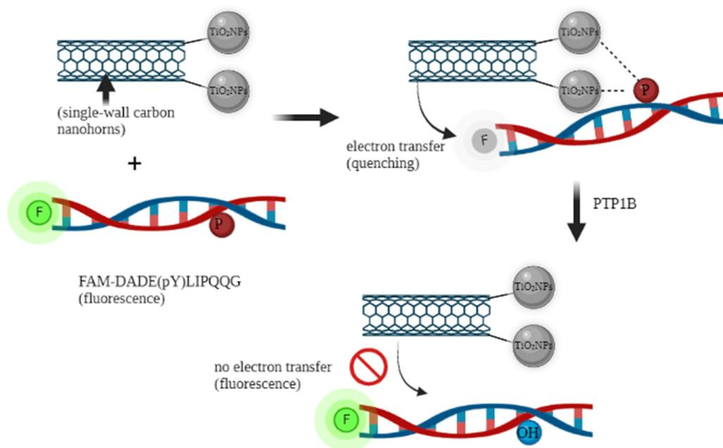
Fig. 6 Modified TiO<sub>2</sub>NP single-wall carbon nanohorns (TiO<sub>2</sub>-SWCNHs) for detecting the tyrosine phosphatase 1B protein (PTP1B). Adapted with permission from ref. 13. Copyright 2022 Elsevier.
