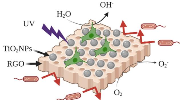
Fig. 7 The graphene oxide/titanium dioxide (RGO@TiO<sub>2</sub>) nanohybrid as a filler to investigate their synergistic effects on electrospun regenerated silk fibroin (RSF) mats. Adapted with permission from ref. 280. Copyright 2021 Elsevier.
