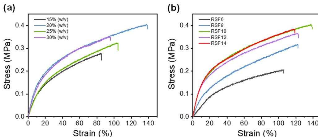
Fig. 3 Typical stress–strain curves of wet RSF films prepared at (a) different  $(\text{NH}_4)_2\text{SO}_4$  concentrations ranging from 15% (w/v) to 30% (w/v) and (b) different SF concentrations ranging from 6 wt% to 14 wt% (20% (w/v)  $(\text{NH}_4)_2\text{SO}_4$  solution).
