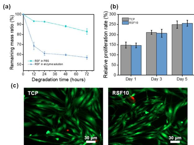
Fig. 5 (a) Weight change of RSF10 in a PBS buffer (pH 7.4) and in protease XIV solution over time. (b) CCK-8 assay of cells' viability on the RSF10 and TCP for 5 day co-culture. Values are means  $\pm$  SD for each group ( $n = 6$ ). (c) Fluorescence microscopy images of cells cultured on the RSF10 for 5 days.
