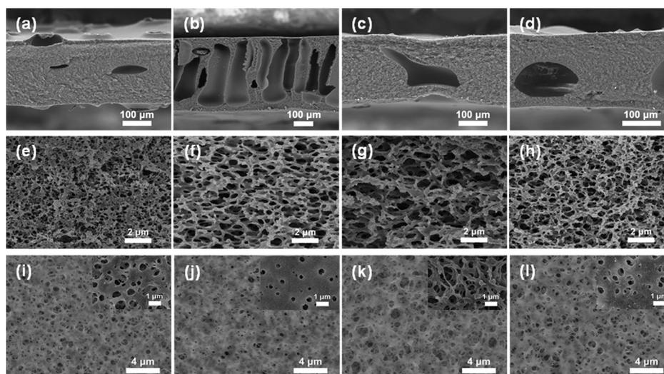
Fig. 2 SEM images of the cross sections (a–h) and surface (i–l) of RSF films prepared from 15% (w/v)  $(\text{NH}_4)_2\text{SO}_4$  solution (a, e and i), from 30% (w/v)  $(\text{NH}_4)_2\text{SO}_4$  solution (b, f and j), and from 6 wt% SF concentrations (c, g and k) and 10 wt% SF concentrations (d, h and l) (20% (w/v)  $(\text{NH}_4)_2\text{SO}_4$ ).
