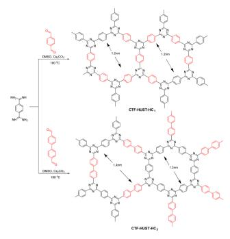
Fig. 15 Synthesis of CTF-HUST-HC<sub>1</sub> and CTF-HUST-HC<sub>2</sub>.
