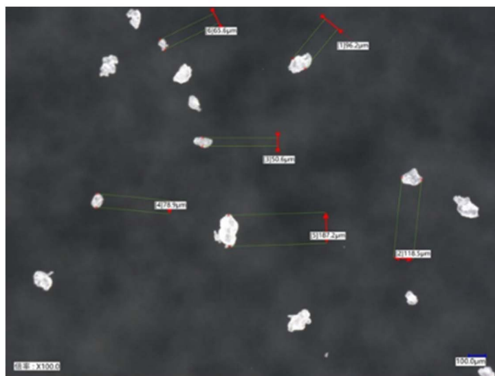
Fig. 37 Biomass biodegradable resin powder. (Top left) PLA base, (Top middle) starch base and (Top right) cellulose base. Optical microscopic observation of PLA-based 100% biomass biodegradable resin powder (Below).
