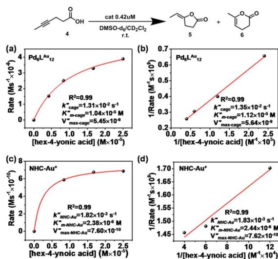
Fig. 7 Kinetic experiments and implications in the cyclization reaction of hex-4-ynoic acid. (a) Kinetic analyses and (b) Lineweaver–Burk plot for the  $\text{Pd}_6\text{L}^{\text{Au}}_{12}$  cage. (c) Kinetic analyses and (d) Lineweaver–Burk plot for  $\text{NHC-Au}^+$ .
