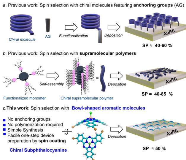
**Fig. 1** Existing strategies to prepare well-ordered chiral assemblies for mc-AFM measurements: (a) formation of SAMs. (b) Deposition of supramolecular polymers. (c) Methodology reported in this work: spin-coating deposition of bowl-shaped SubPcs (atom's colour code: carbon in turquoise, nitrogen in blue, hydrogen in white, boron in pink, chlorine in green and bromine in orange).
