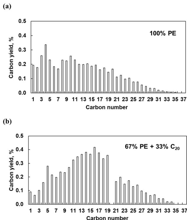
Fig. 12 Carbon yield as a function of the product carbon number for liquid and gaseous products formed from pure PE (a) and PE mixed with C<sub>20</sub> *n*-alkane in a 67 : 33 wt% proportion (b). Reaction conditions: 300 °C, 30 bar H<sub>2</sub>, 5 h reaction time, 6.4% Pt/Al<sub>2</sub>O<sub>3</sub> 0.1 g, 2 g PE or 1.32 g PE mixed with 0.67 g C<sub>20</sub>.
