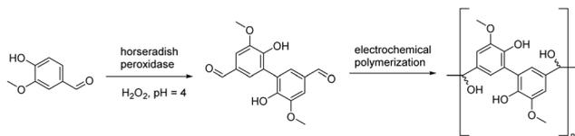
**Scheme 6** Electrochemical synthesis of polyvanillin via the reductive coupling of divanillin.
