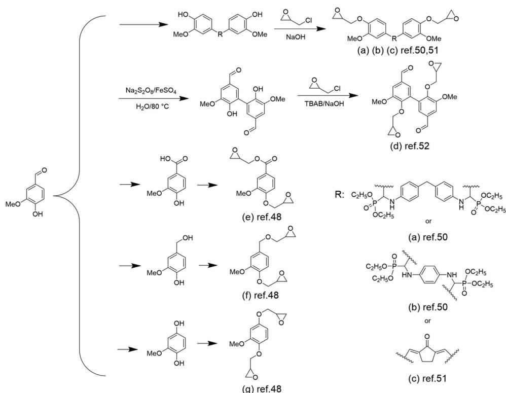
**Scheme 2** Overview of the synthetic route of vanillin-based epoxy monomers: (a) and (b) Reproduced from ref. 50 with permission from the American Chemical Society, copyright 2017. (c) Reproduced from ref. 51 with permission from Elsevier, copyright 2017. (d) Reproduced from ref. 52 with permission from the American Chemical Society, copyright 2020. (e), (f) and (g) Reproduced from ref. 48 with permission from Elsevier, copyright 2015.
