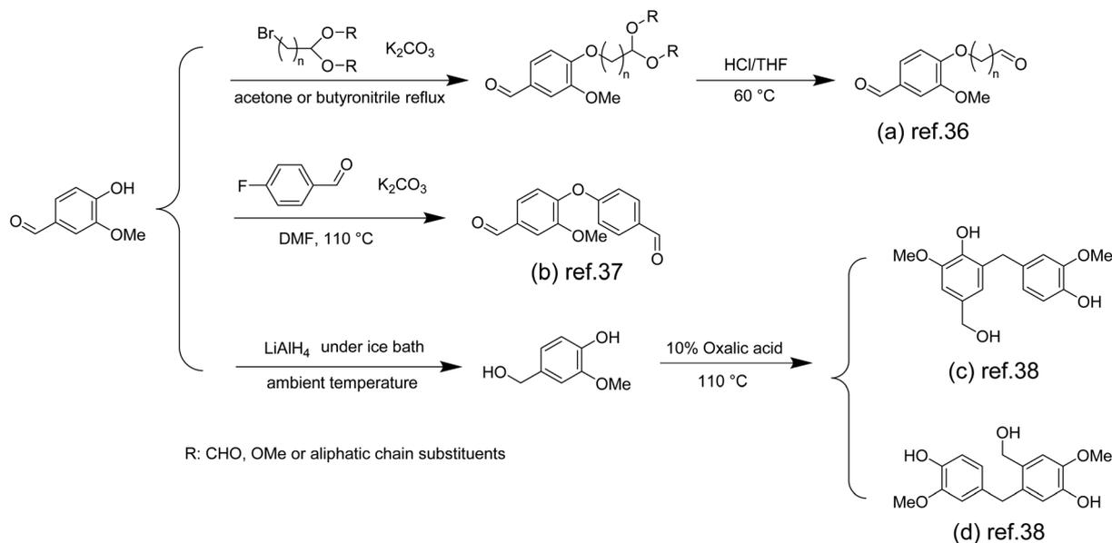
**Scheme 1** Overview of the preparation route for monomers used in the synthesis of phenolic resins: (a) Reproduced from ref. 36 with permission from Elsevier, copyright 2016. (b) Reproduced from ref. 37 with permission from Elsevier, copyright 2016. (c) Reproduced from ref. 38 with permission from Elsevier, copyright 2021.
