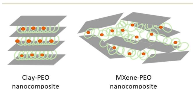
Fig. 9 Structural arrangements of clay-PEO based on montmorillonite layered clay mineral, described by Ruiz-Hitzky and Aranda,<sup>233</sup> and MXene-PEO based on Ti<sub>3</sub>C<sub>2</sub>T<sub>x</sub>, described by Pan *et al.*<sup>243</sup>
