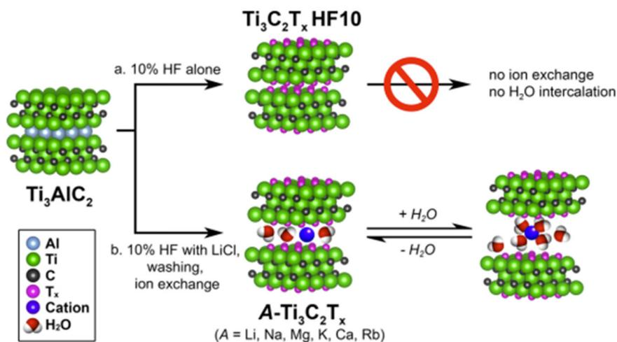
Fig. 5 Scheme showing the preparation of MXenes from the  $Ti_3AlC_2$  MAX phase etched with (a) 10% HF alone (which does not intercalate cations and water molecules), and (b) 10% HF in the presence of LiCl (leading to  $A-Ti_3C_2T_x$  materials possessing ion-exchange and reversible  $H_2O$  adsorption properties in the interlayer space). Reprinted with permission from Ghidui *et al.*, *Chem. Mater.*, 2016, 28(10), 3507–3514. Copyright 2016 American Chemical Society.
